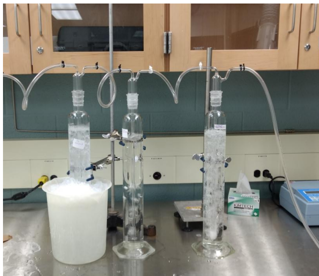
Figure 3.2 Bench Scale Set-Up Generating an Ozone Stock Solution. The first wash bottle contains a bubble diffuser and was used to create the ozone stock solution. The next two bottles are filled with quenching solutions. The second bottle was the only bottle that did not contain a bubble diffuser.
