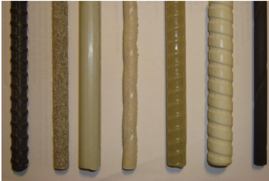
Figure 2.3 Different types of FRP bar/tendon (Quayyum, 2010)
