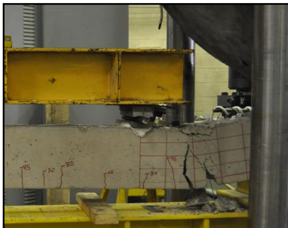
b) Prestressed beam after failure
