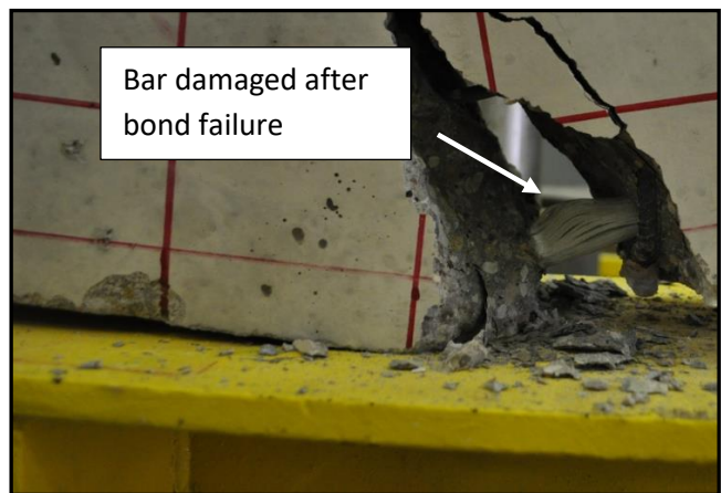
a) Prestressed GFRP bar after failure
