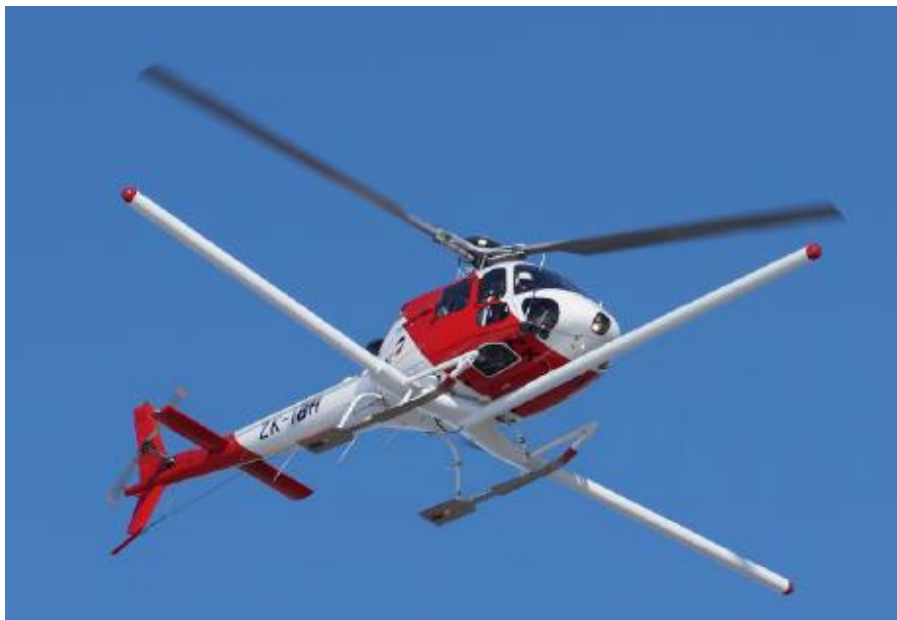
Figure 4.3: Airborne radar system designed by UTIG and mounted on an AS-350 helicopter. The left and right boom contained the two independent pairs of radar antennas, the front boom was empty. Photograph by UTIG 2017 field participants.
