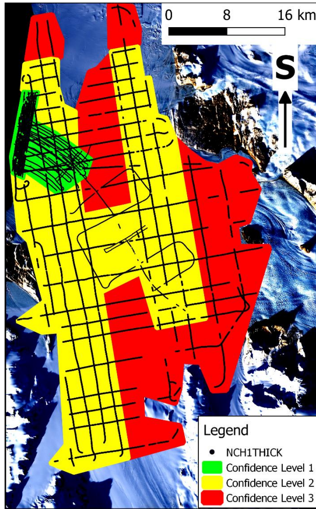
Figure 4.5: Sectors of confidence level within the main NIS extent. Confidence level 1, 2 and 3, have ice thickness data densities of 618, 80 and 35 ice thickness values per \text{km}^2 respectively.
