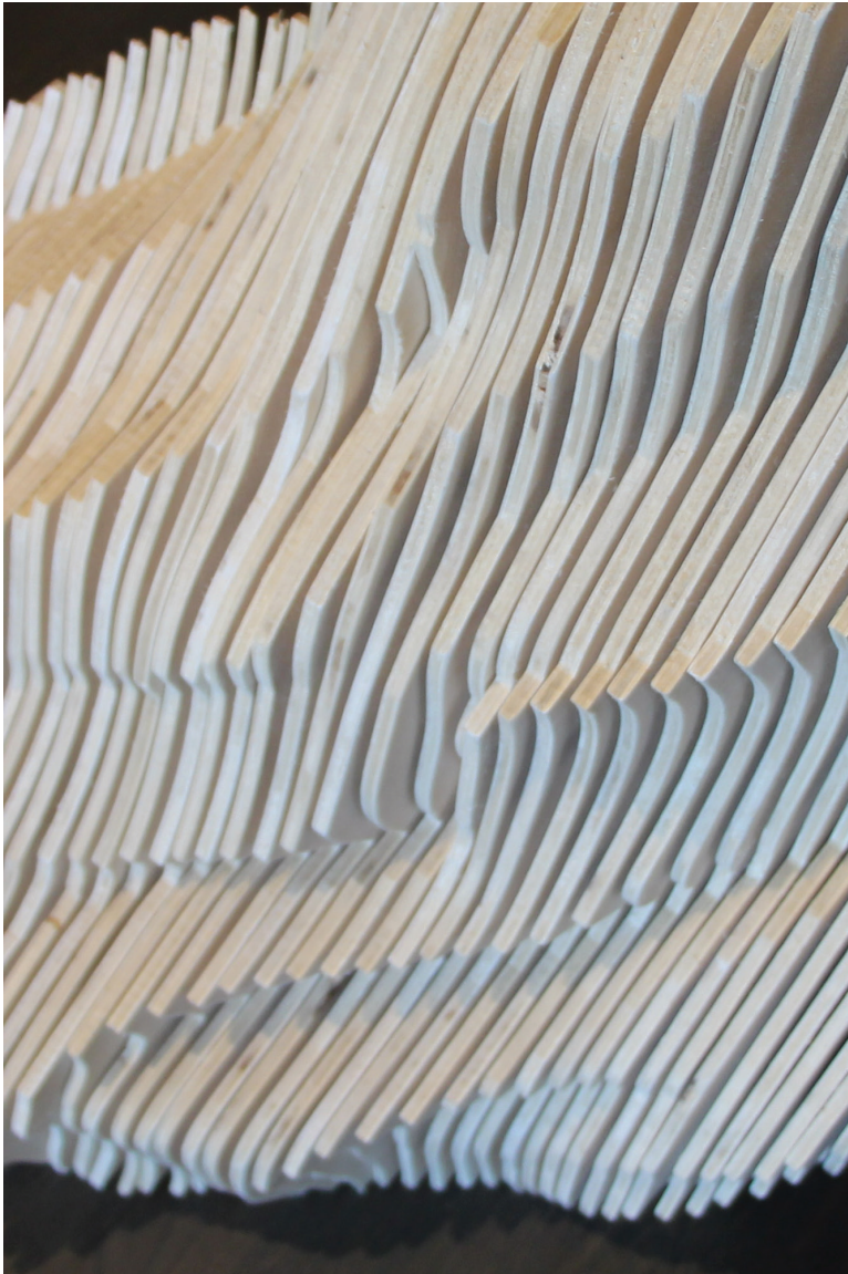
FIG 4.33 DETAIL OF 1:2.5 SCALE MODEL OF TOP PIECE IN PLYWOOD.
