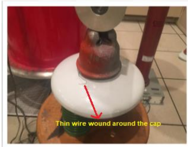
Fig.3.3. Hardware corona generated using a thin wire wound around the cap of a line insulator.
