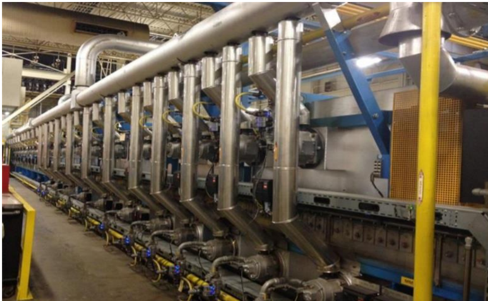
Figure 5: Continuous roller hearth furnace, located at Formet Industries, St. Thomas, ON. The furnace is used for austenitizing blanks and transforming the as-received eutectic coating to an intermetallic Al-Si-Fe layer during heating.
