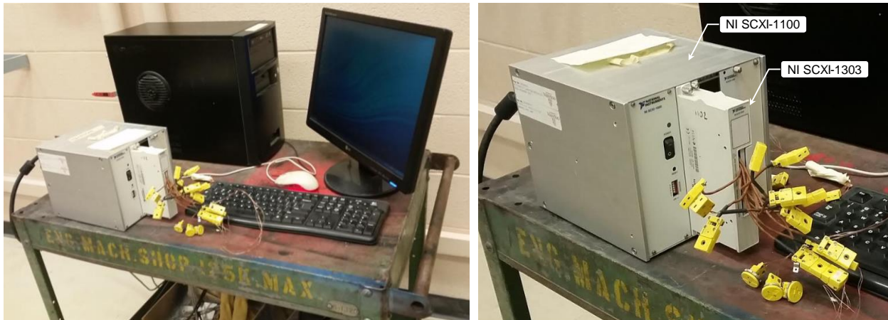
Figure B1.1: Equipment setup used for the laboratory muffle furnace. National Instruments SCXI-1000 chassis used with SCXI-1303 32-channel terminal block for thermocouple connection.
