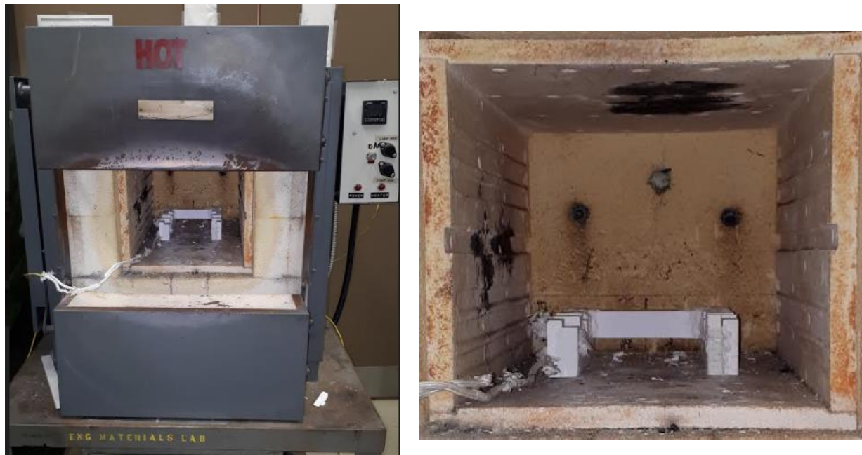
Figure 16: Thermolyne™ lab scale muffle furnace utilized for in-house heat treatment. This furnace was further used to validate the thermometallurgical model, discussed in Chapter 4.
