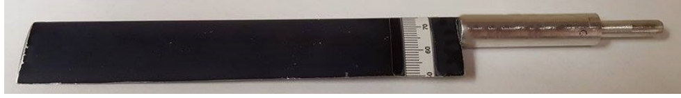
Figure 2.4: Manufactured SD7037 airfoil model.
