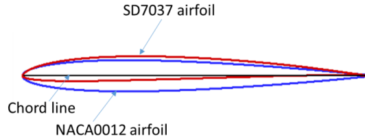
Figure 2.3: Schematic of the SD7037 airfoil compared with NACA0012.
