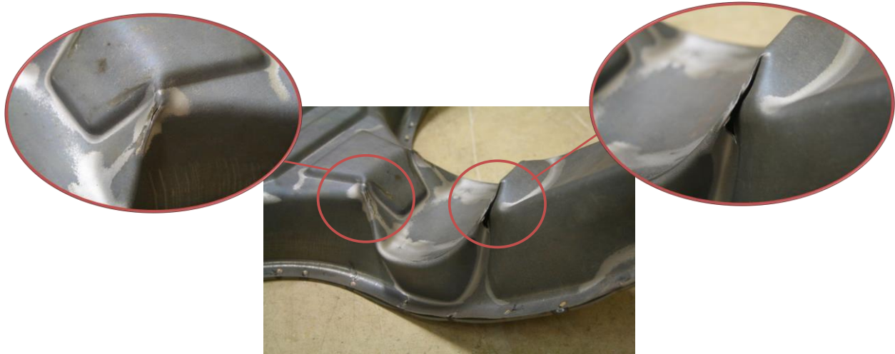
Figure 17 Failed specimen from side impact test (Figure 16). Cracks were observed at the edge of the impact zone where severe local folding exists.
