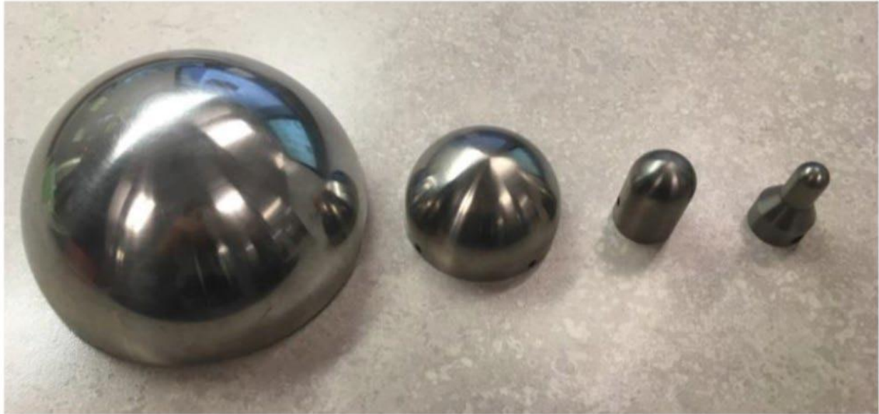
Figure 74 Hemispherical dome punches. From left to right: 50 mm, 25 mm, 10 mm, and 5 mm in radius
