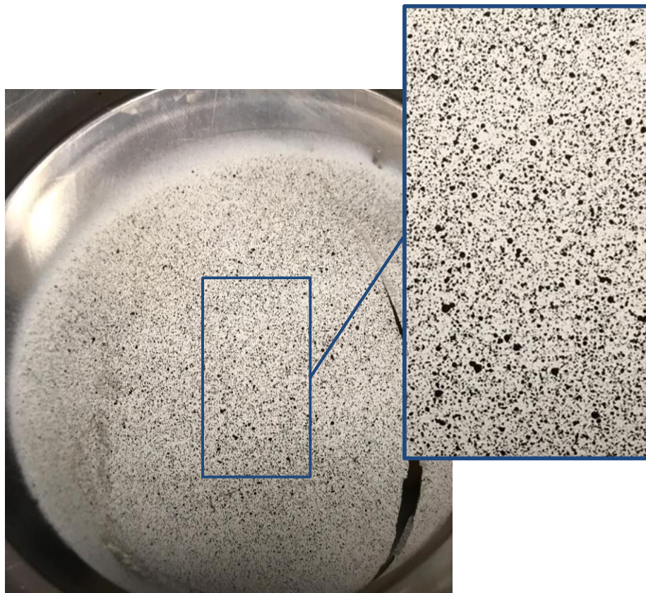
Figure 23 Randomized speckle patterns to help DIC for tracking of local deformation for a Nakazima dome test specimen. The optimal size of the speckle may vary depending on the test setup
