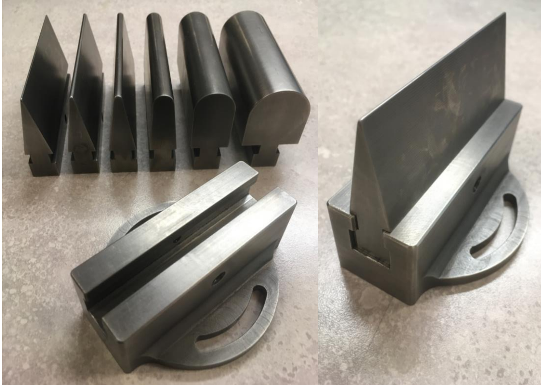
Figure 87 Stretch-bend punches with different radii (left) from left to right: 0.4, 1, 2, 5, 10, and 15 mm in radius. Smaller punch radius corresponds to the higher bend severity. Punch assembled to the holder (right)
