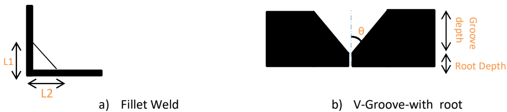
Figure 43 Weld joint geometry configuration
