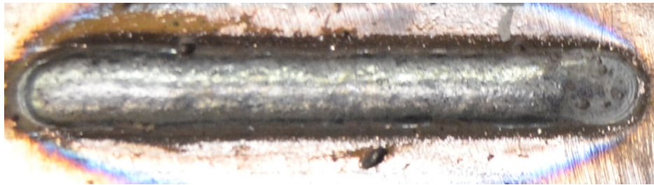
Figure 5 Weld bead made by Gas Metal Arc Welding
