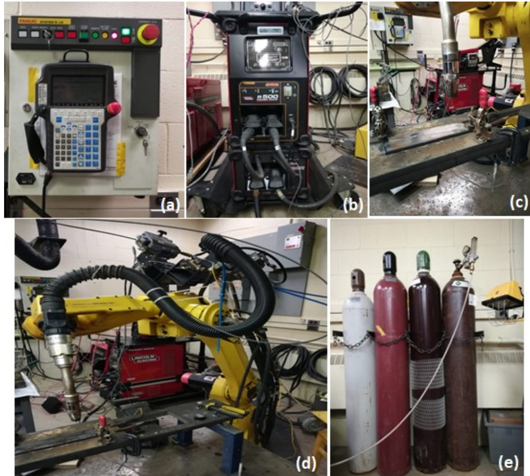
Figure 17 Welding System (a) FANUC R3J Controller; (b) Lincoln Electric™ R500 Power Supply; (c) Bead on Plate Setup; (d) FANUC Arcmate i120c automatic welder robot; (e) Gas Cylinders with flow meter
