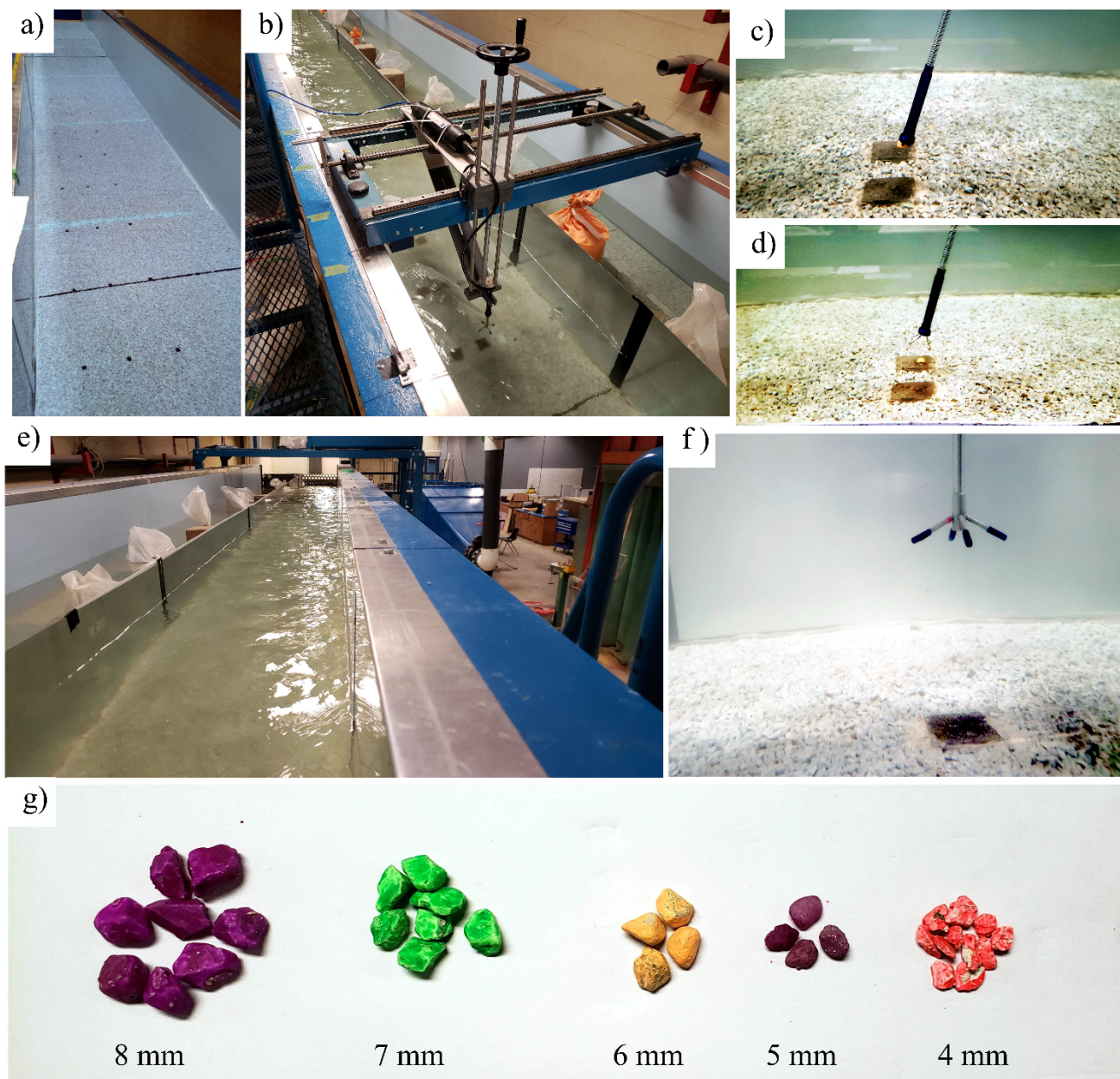
Figure 5-2 experiment apparatuses, a) The flume bed and riffles are covered with roughness mats, b) the probe holder trolley for Vectrino II, c, and d) placing a particle on the test pad using a bolt grabber, e) looking upstream of the flume that is narrowed by false walls, f) the Vectrino II probe measuring velocity profile, g) different sizes of painted particles
