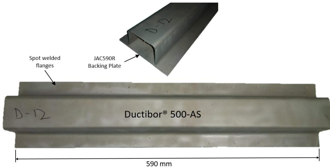
Figure 70: Welded side impact beam specimen with coating removed by sandblasting.
