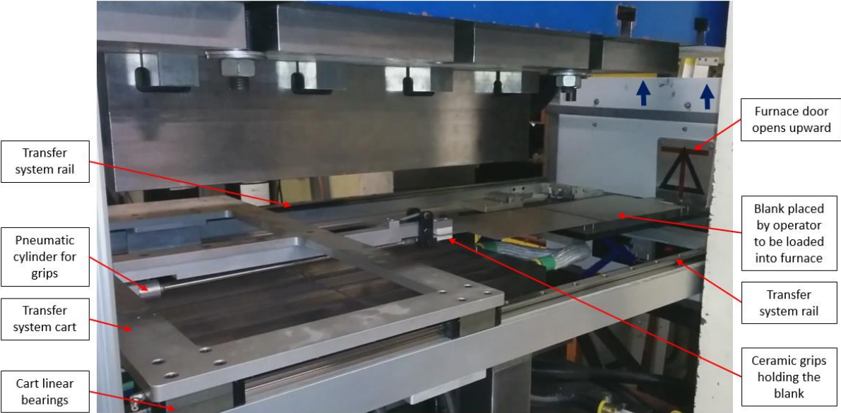
Figure 61: Transfer system in press with furnace and rail die, blank is loaded.
