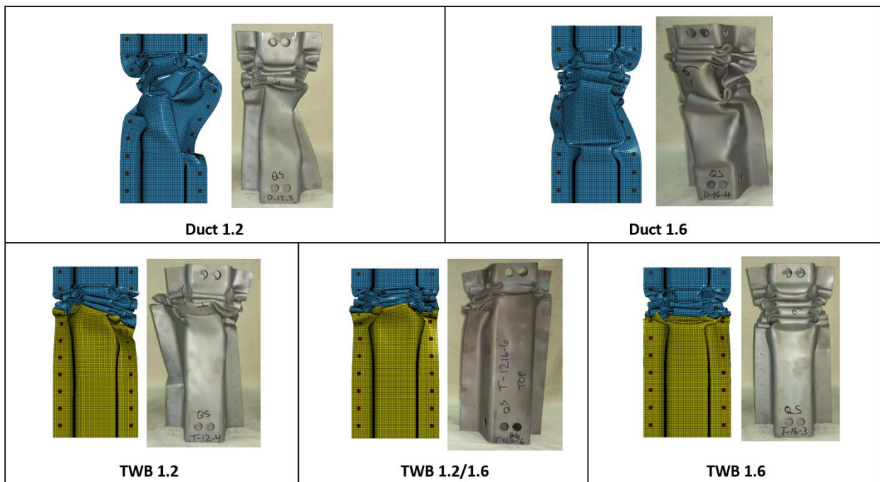
Figure 175: Comparison of deformation modes in quasi-static axial crush experiments and models for each material condition.
