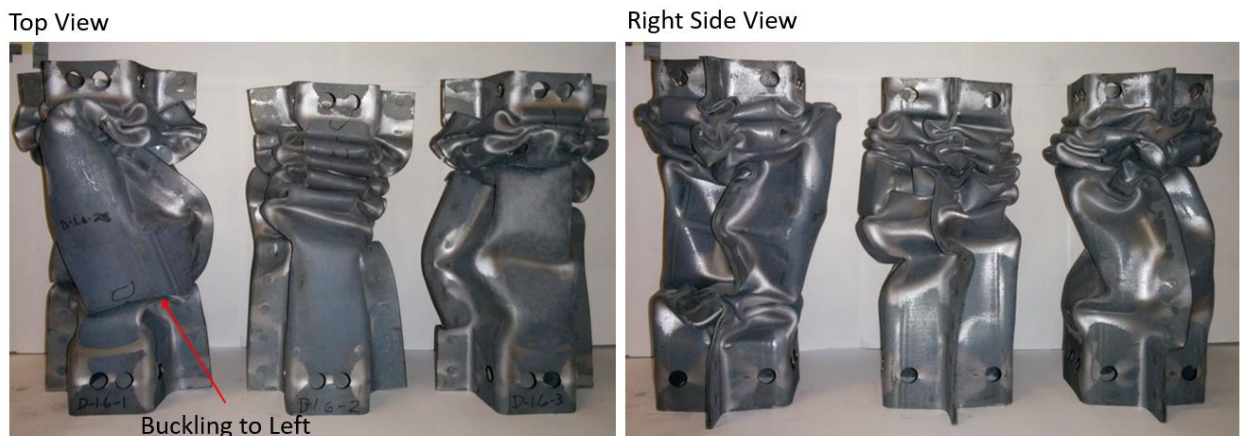
Figure 140: Final shape of three 1.6 mm Ductibor® 500-AS specimens after dynamic crush.
