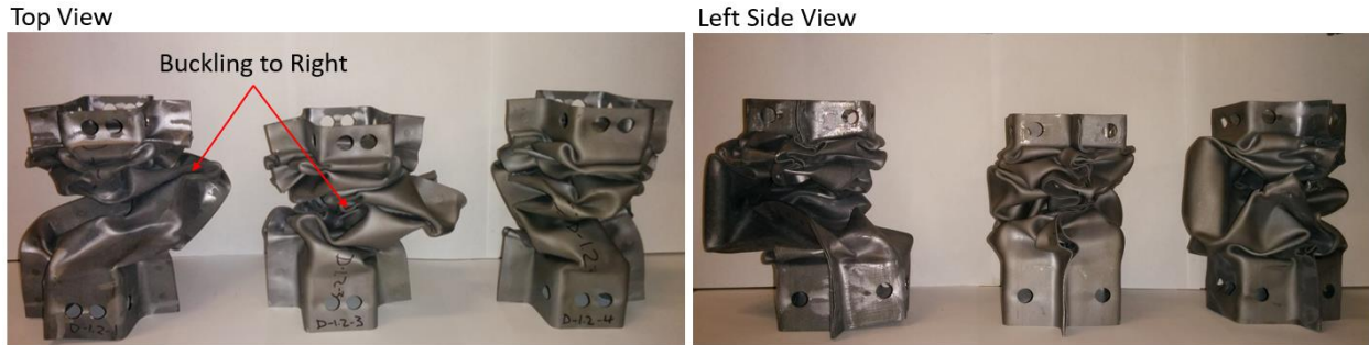
Figure 137: Final shape of three 1.2 mm Ductibor® 500-AS specimens after dynamic crush.
