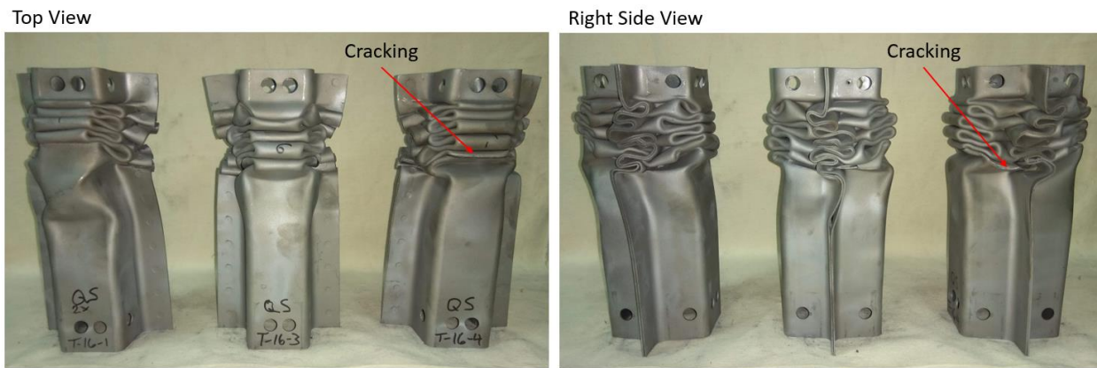
Figure 169: Final shape of three 1.6 mm TWB specimens after quasi-static crush.
