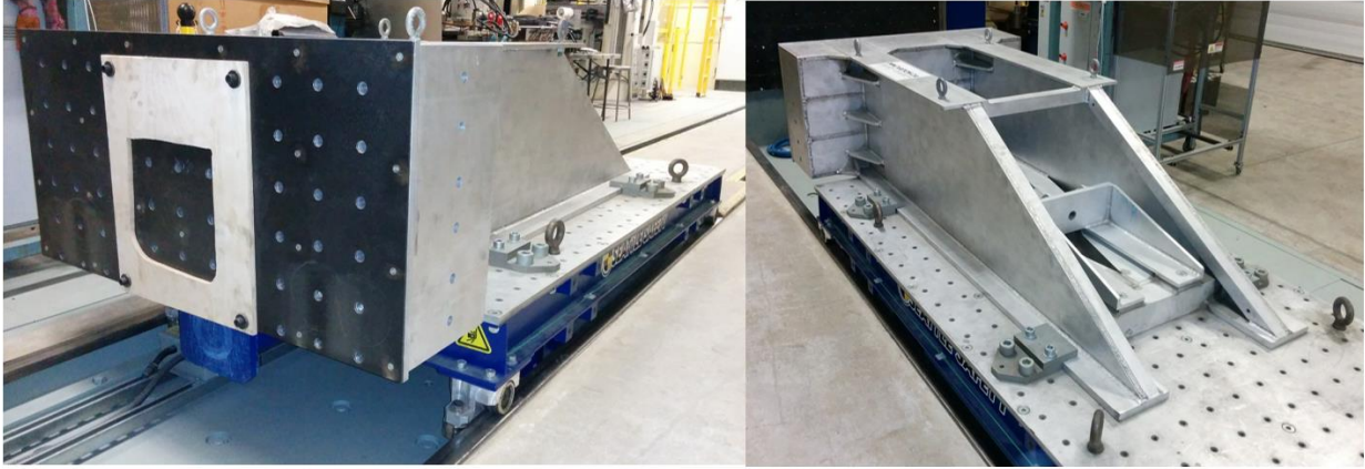
Figure 76: UW Seattle Safety crash sled used for smaller test articles in this thesis.
