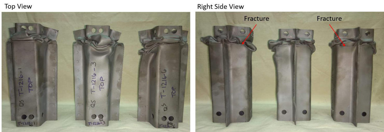
Figure 166: Final shape of three 1.2/1.6 mm TWB specimens after quasi-static crush.
