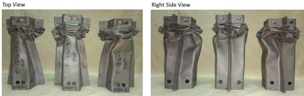
Figure 147: Final shape of three 1.2/1.6 mm TWB specimens after dynamic crush.
