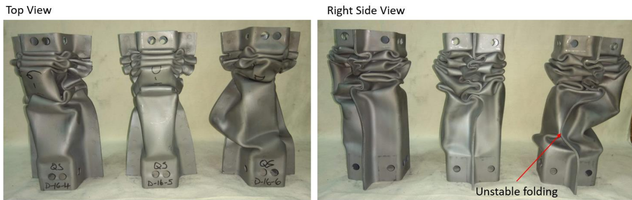
Figure 160: Final shape of three 1.6 mm Ductibor® 500-AS specimens after quasi-static crush.
