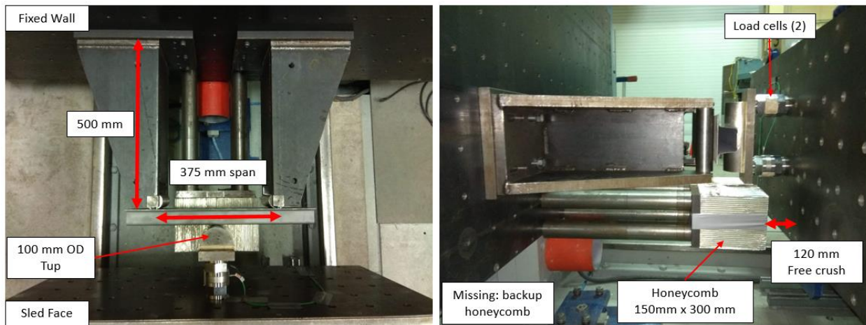
Figure 78: Dynamic three point bend support setup.
