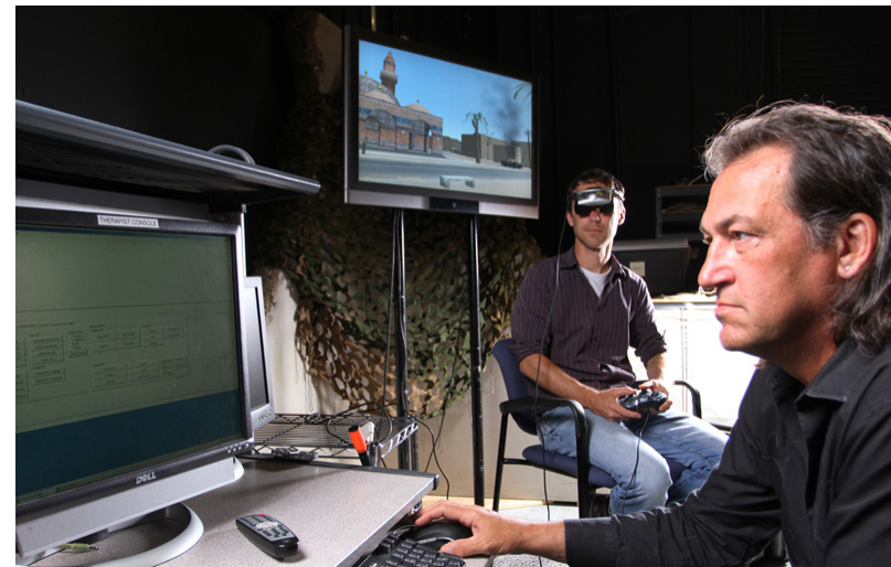
Figure 2.6 The dashboard adds or removes individual sensory stimuli into the VR experience, allowing granular control over the therapy session.
