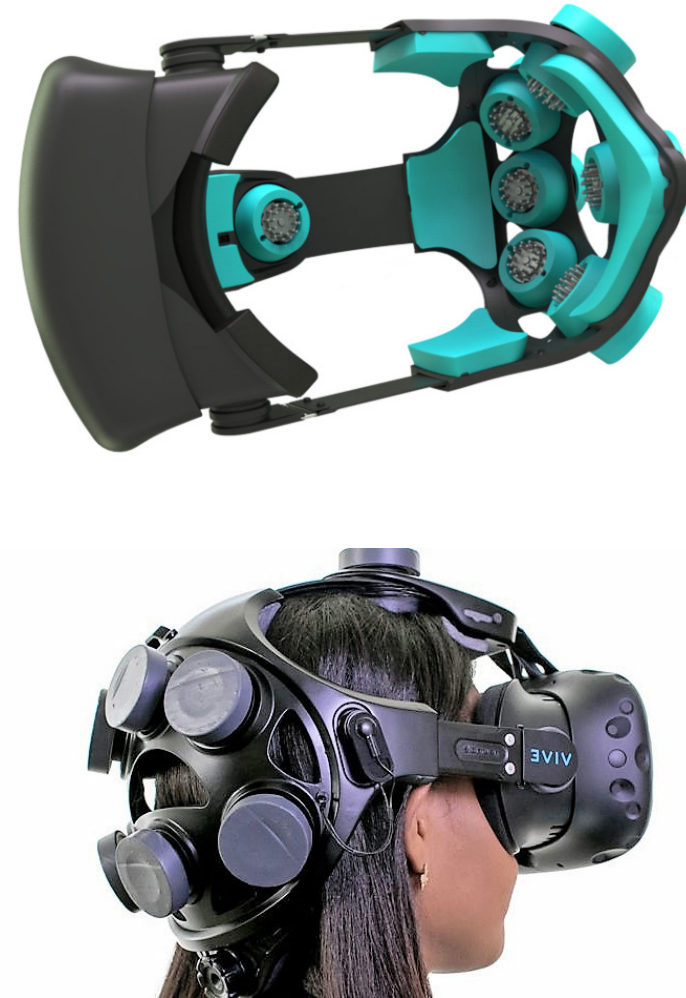
Figure 7.3 The Neurable EEG headset that is designed to attach to the HTC Vive.
