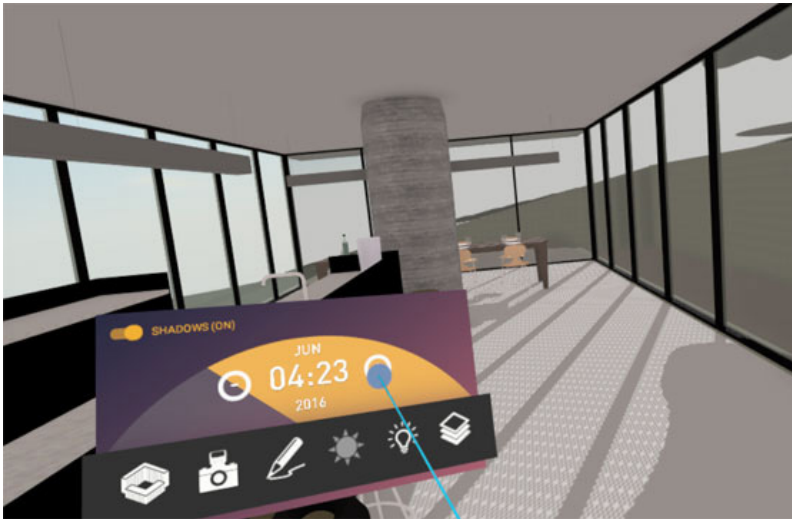
Figure 0.5 With software like IrisVR, architects can take a 3D model and view it in VR within a matter of seconds.
