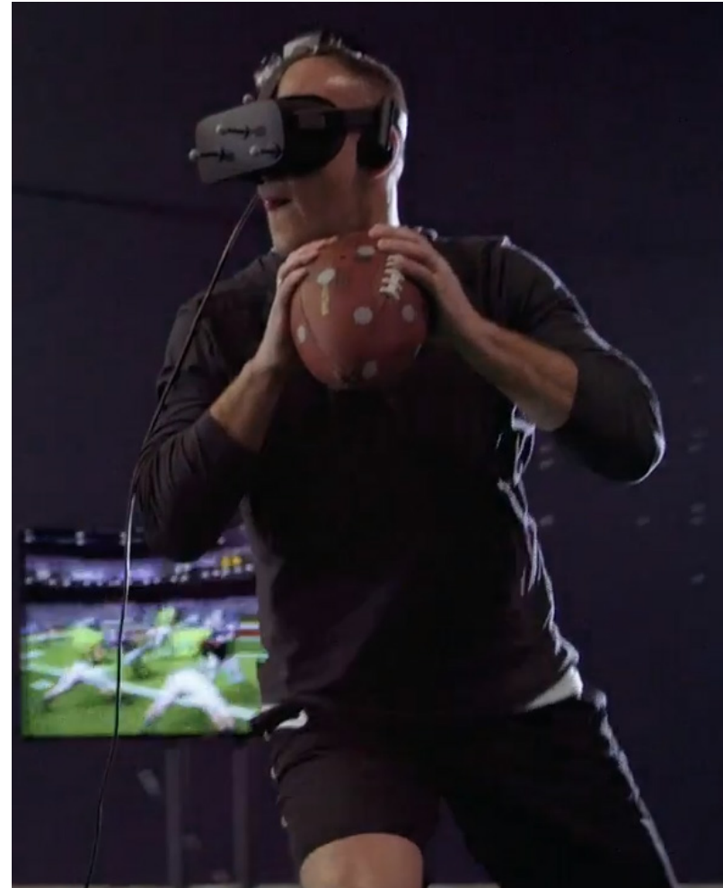
Figure 0.9 QB Sim, a football training VR system that tracks the ball as well as the user, enabling players to practice their passing mechanics in a VR environment that is set up to mimic “game-day” intensity levels. The focus of the training is to familiarize players with different formations that the opposing team might utilize, so that they can predict what might happen based on how opposing players line up.
