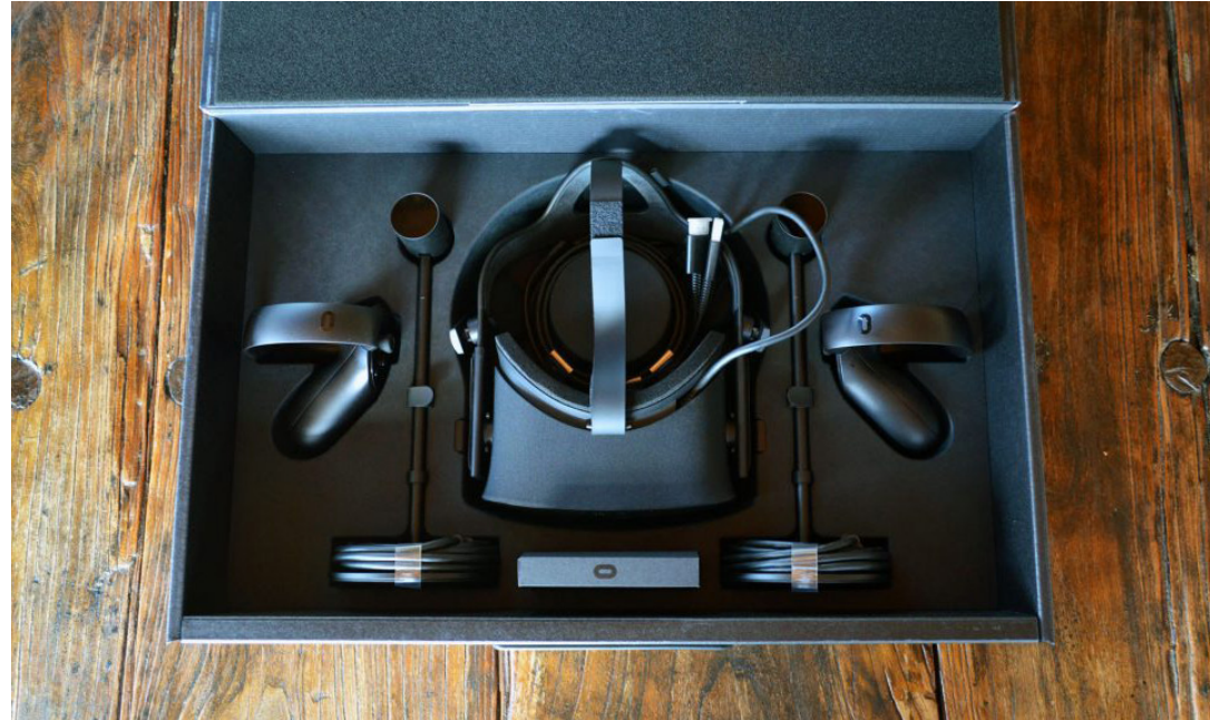
Figure 4.2 The different components of the Oculus Rift VR system; starting from the center is the Oculus Rift headset, then the infrared sensors that track the user's movements, and on the outside are the Oculus Touch controllers.
