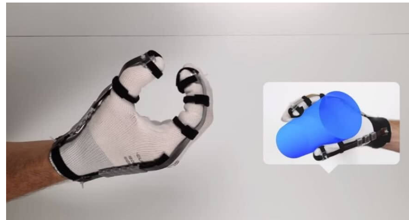
Figure 2.11 VR gloves that prevent the fingers from bending past a certain point when the user grasps an object in VR, giving the sensation of holding a physical object.
