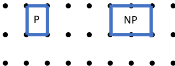
FIGURE 2.2: Examples of a primitive unit cell (left) and a nonprimitive unit cell (right). P = primitive unit cell; NP = nonprimitive unit cell.
