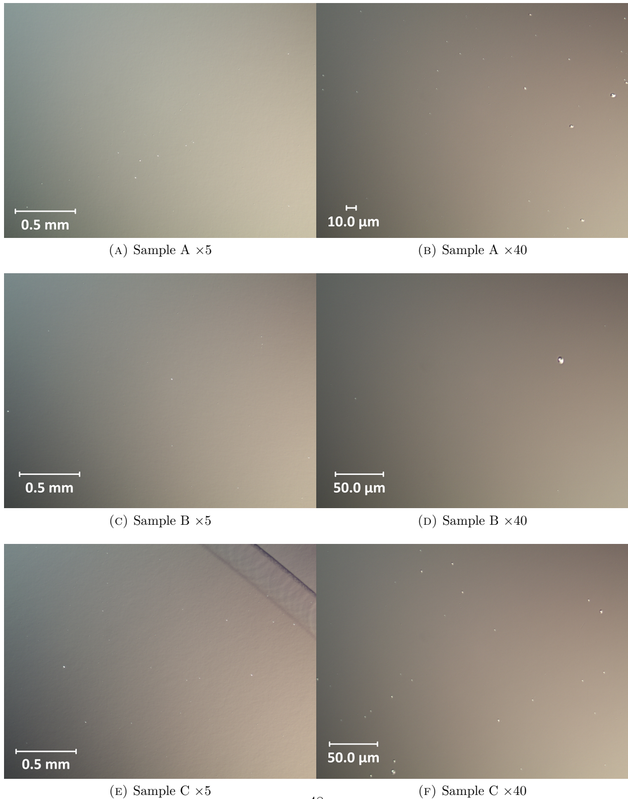
FIGURE 7.1: Nomarski images for Sample A, B, and C at \times 5 and \times 40 magnifications
