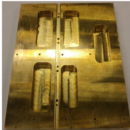
Figure 4.19: Photograph of the base with balun cavities.
