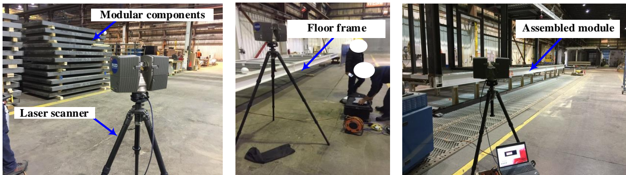
Figure 5.9. Application of laser scanning technology for real-time data collection.
