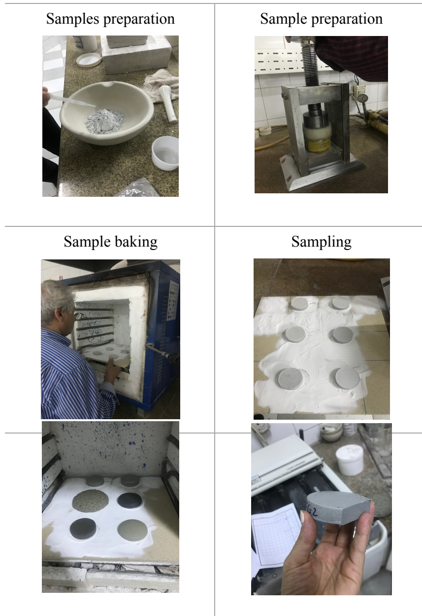
Figure 3: Sampling steps for Foam-Glass Lightweight Aggregate (FG-LWA) (Foamyna Canada Inc)
