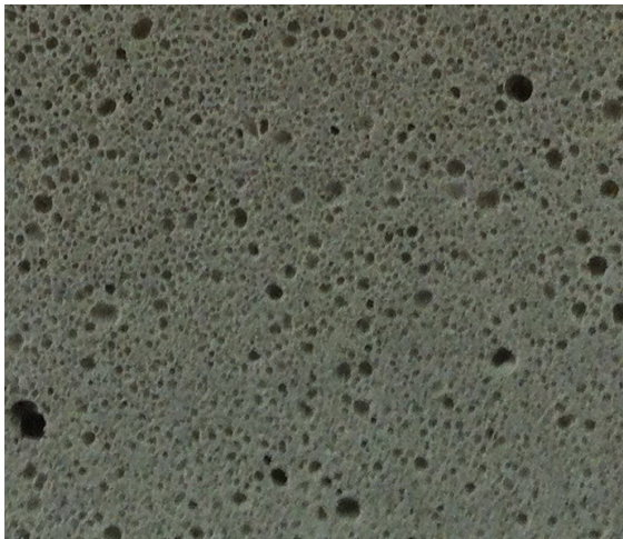
Figure 8: Foam Glass containing waste frit
