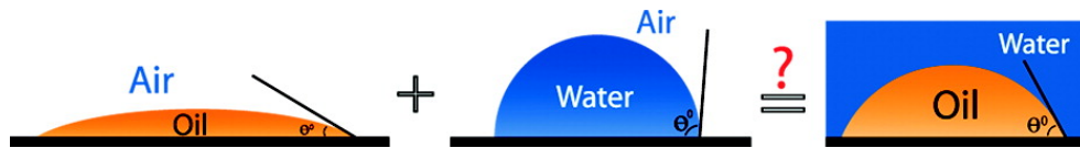
Figure 2.2: Schematic representation by Goossens et al. [18] to establish a link between the dynamics of wetting in liquidliquid and in liquidair systems. Image is reproduced with permission from ACS Publications
