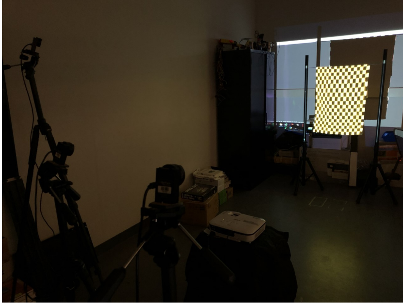
Figure 5.8: Photo of experimental setup with motion capture cameras, a projector and a towel being projected onto.
