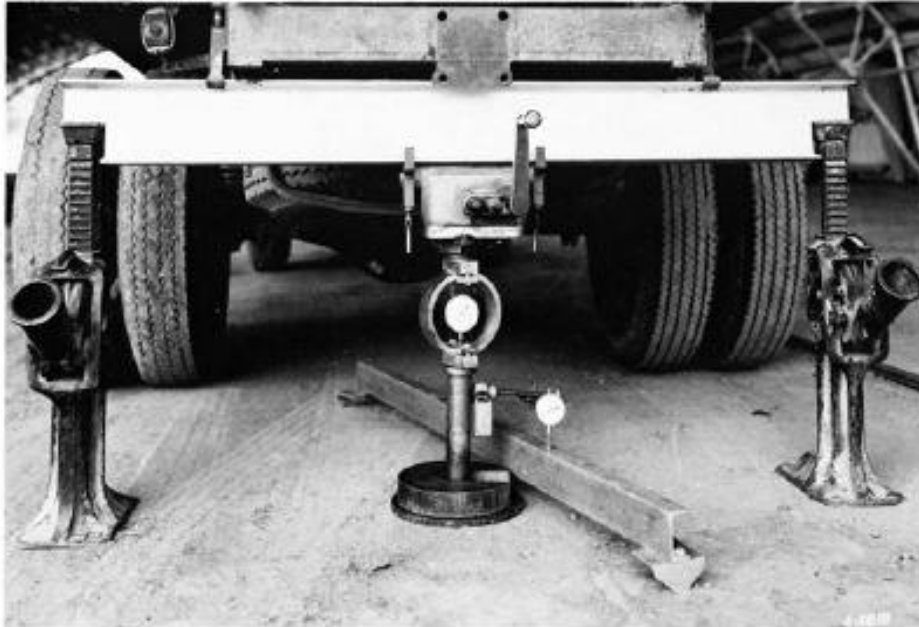
Figure 2.2: Example of field in place testing setup (ASTM D4429, 2009)
