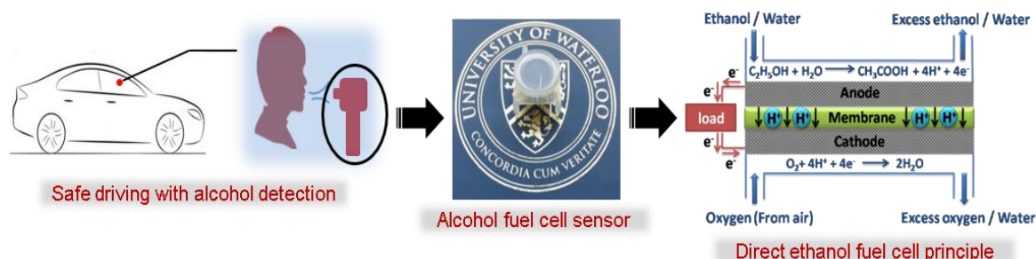
Figure 5-1. Schematic diagram of an AFCS and its electrochemical principle.
