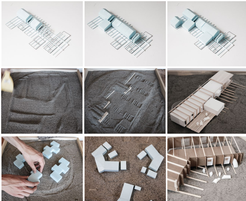
f 1.27 Breaking apart the Five-plex. Various model studies of the typical Five-plex housing type. Growing the Five-plex over time (top); earthwork and foundation studies (middle); facade and massing studies (bottom).
