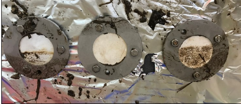
Figure D-4 – Three POCIS removed from the stream (SA-DS) after a 14-day deployment. The POCIS may have been exposed to the air during a portion of the deployment period, as shown by the inconsistent lines and fouling on the membranes. Photos taken by Maria Digaletos (2017).
