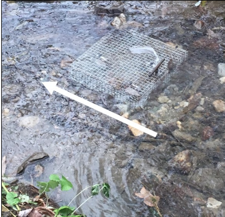
Figure D-3 -Placement of the passive samplers within a wire cage in a stream (SA-DS). The membranes of the POCIS and P-Traps are placed parallel to the flow of the stream to allow interaction with both sides of the samplers. Photos taken by Maria Digaletos (2017).
