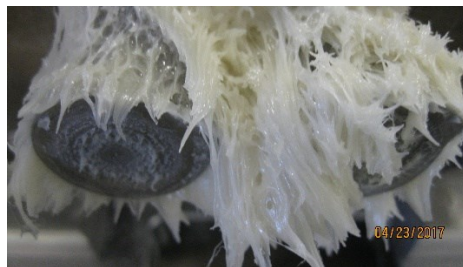
Figure 3-3 Thermoplastic starch covered Banbury rotors
