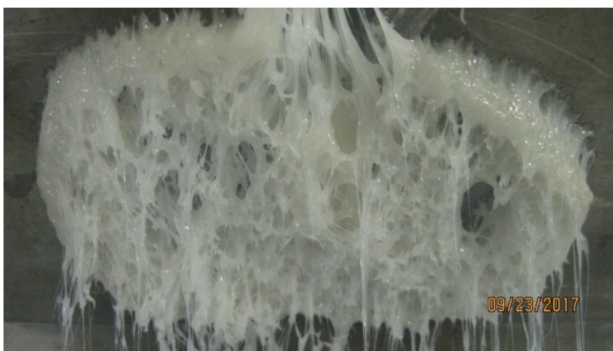
Figure 3-1 View of thermoplastic starch on rotor of the CWB mixer on opening
