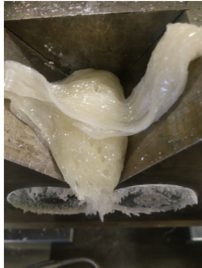
Figure 4-13 Photograph of the polymer melt with gas bubbles present
