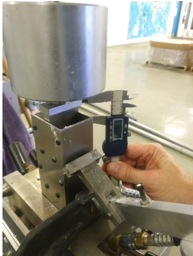
Figure 4-12 Photograph depicting the loading chute ram and weight raised above the neutral position displayed at charge.
