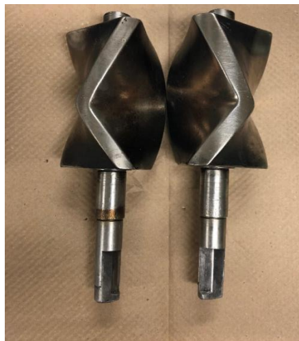
Figure 3. 2 Haake Rheocord 90 batch mixer with rotors.
