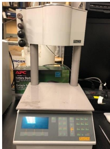
Figure 3. 6 Dynisco D4002 melt flow indexer.
