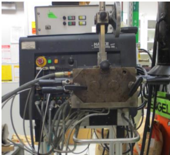
Figure 3. 2 Haake Rheocord 90 batch mixer with rotors.
