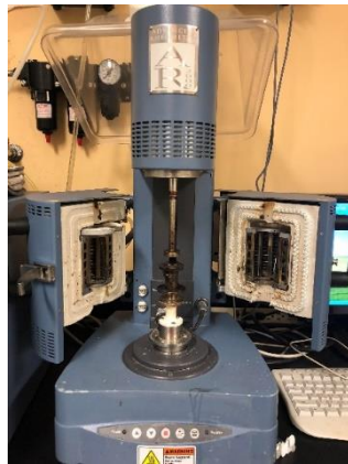
Figure 3. 5 TAI AR2000 rotational rheometer.
