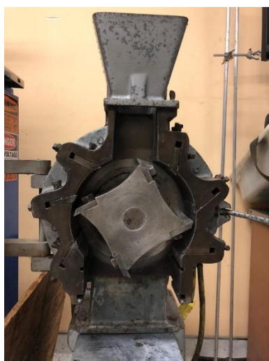
Figure 3. 2 Haake Rheocord 90 batch mixer with rotors.
