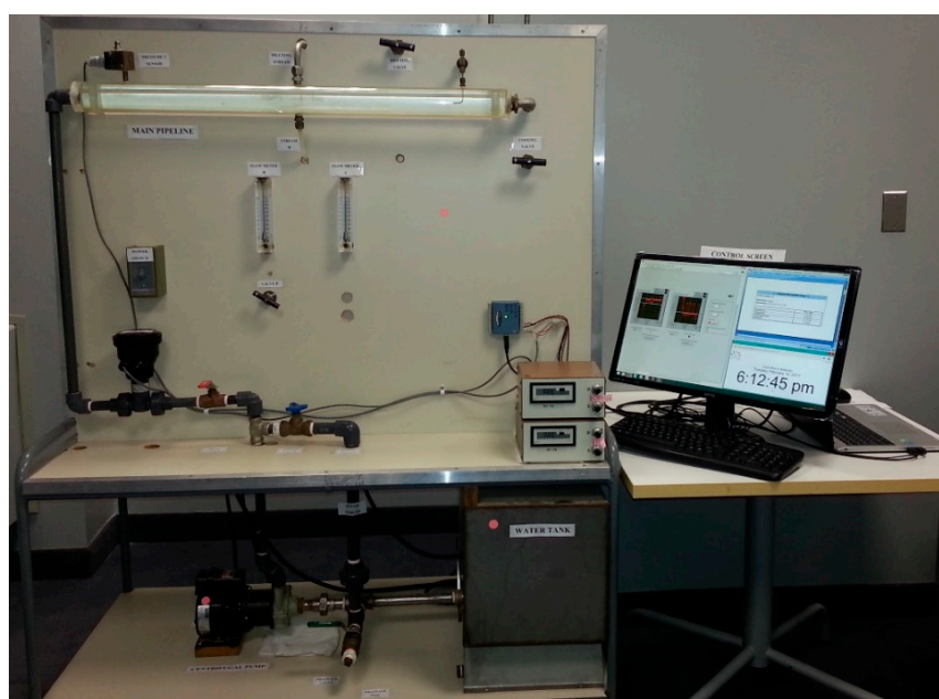
Figure 1. Experimental setup of the hydraulic pump system used in the current study.
