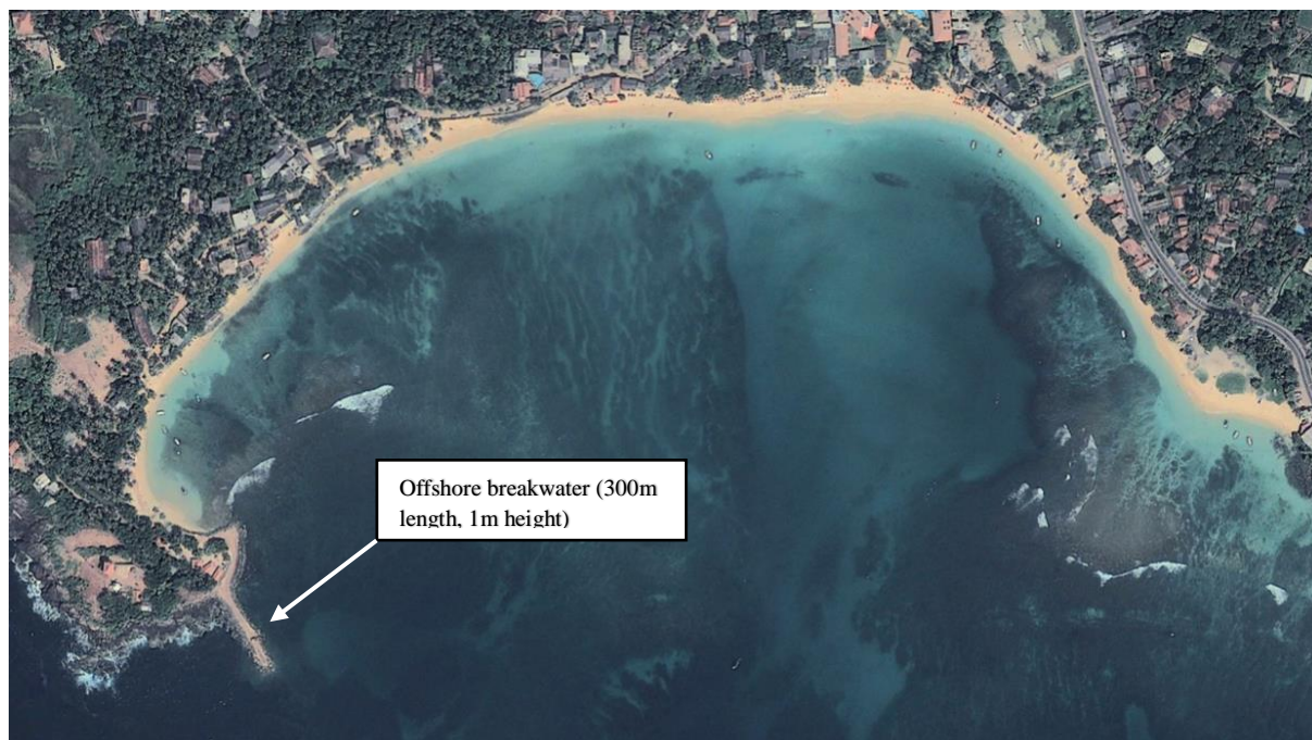
Figure 6.4: Beach profile of Unawatuna from January 13, 2013 following construction of the breakwater
