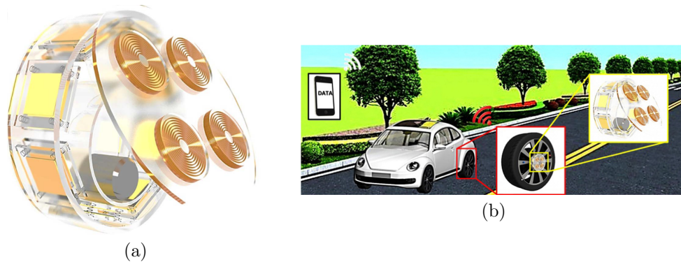
Figure 2.11: (a) Schematic diagram of the designed hybridized generator (b) schematic of the WSN charged by the proposed nanogenerator used in a tire; used with permission [10], Copyright 2017 Elsevier
