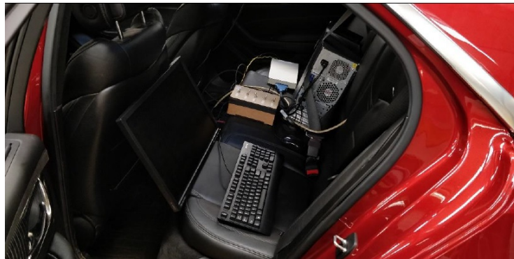
Figure 6.4: Completed in-vehicle data acquisition system
