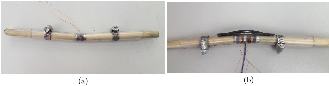
Figure 3.17: Fabricated hybrid electromagnetic-triboelectric generator: (a) single stack (b) double stack
