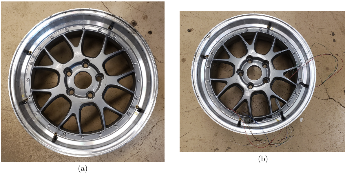
Figure 6.1: Instrumented rim: (a) with modified valves, (b) with wiring
