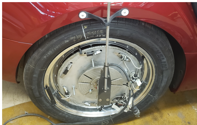
Figure 6.3: The installed smart tire
