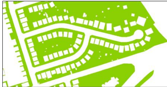
Figure B4.1: An example of a residential area in the GTA. The roads and building footprints were removed to best estimate the remaining area also known as the lot coverage.
