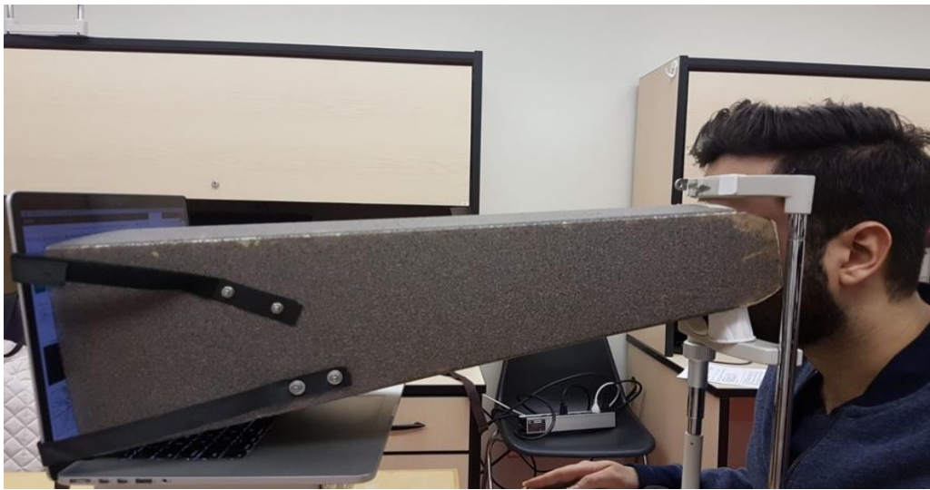
Figure 4-2 Visual tunnel was used during the experiment, allowing a 56.5 cm viewing distance.
