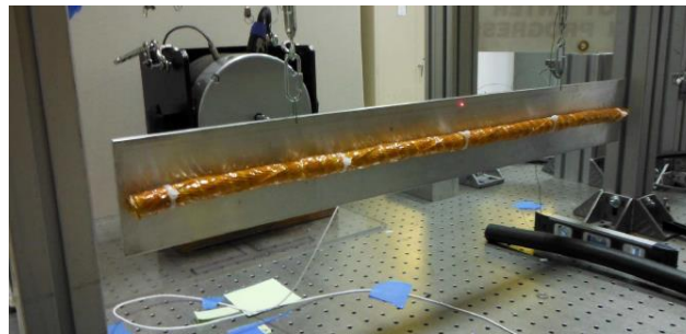
Fig. 1. 8 Cable harnessed structure experimental setup by Inman research group. Courtesy: Spak, PhD thesis, 2014, Virginia Tech [12]
