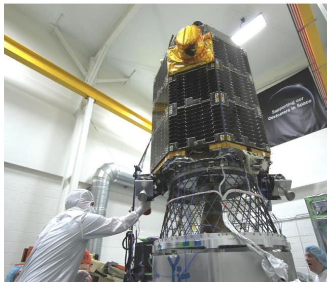
Fig. 1. 3 Setup of NASA Satellite structure on shaker for vibration testing, Image Courtesy: NASA LADEE Website [14].
