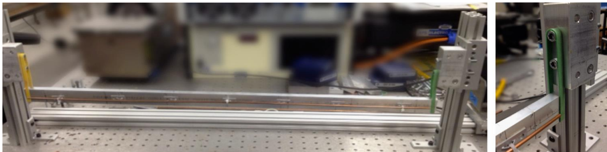
Fig. 1. 9 Cable harnessed structure to validate the spectral element method by Inman research group. Courtesy: Choi et al, JSV 2014 [44]
