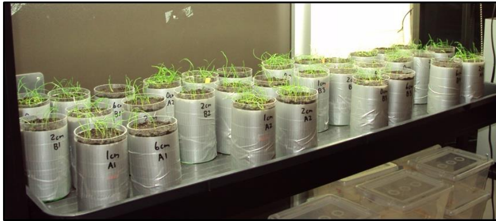
Figure 2.1: Artificial burial cylinders on a plant stand with grass seed artificially sown at different soil depths (0 cm, 1 cm, 2 cm, 6 cm).
