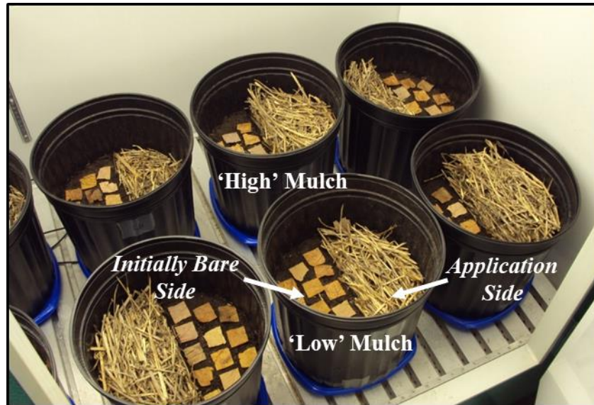
Figure 3.4: Mulch collection microcosms immediately after setup. 12 additional leaf squares beneath mulch amendments not visible. Examples of ‘Low’ ( 2.5 \text{ USG}\cdot\text{m}^{-2} ) and ‘High’ mulch application rates ( 10 \text{ USG}\cdot\text{m}^{-2} ) with different container areas labeled.
