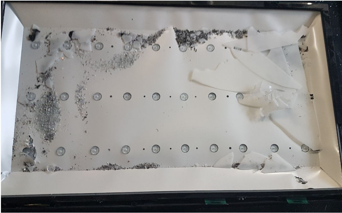
Figure 48 - Chips and Debris from Screen Milling
