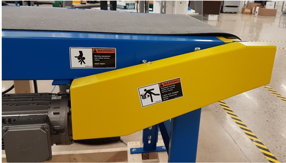
Figure 10 - Conveyor for Automated Loading
