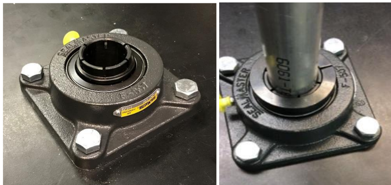
Figure 6.4. Main shaft's bearing installed on the table.
