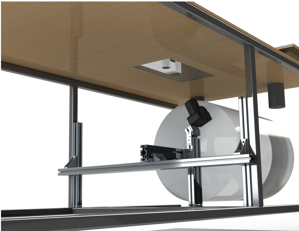
Figure 3.18: A rendering of the camera position and optical rails
