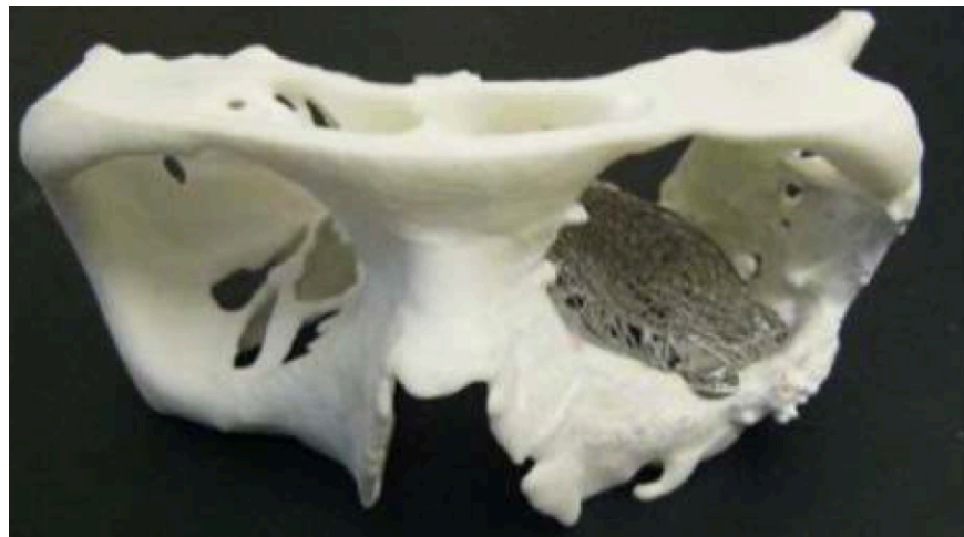
Figure 10: Ti64 reconstruction plate printed by EOS [68].
