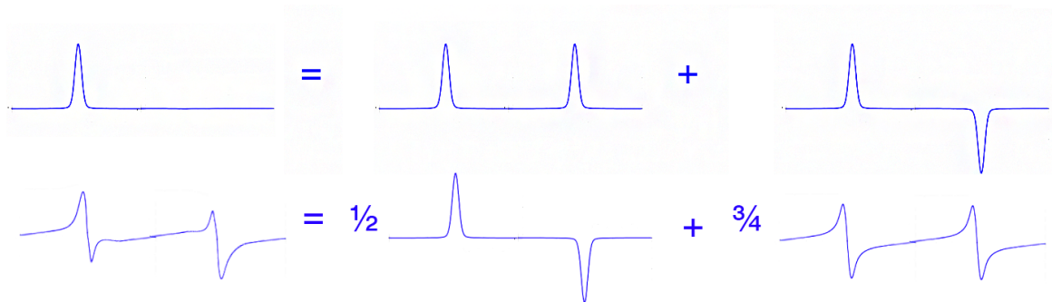
Figure 2.7: An example of two spectra decomposed into linear combinations of the XI , YI , XZ and YZ spectra. The first spectra is equal to XI + XZ while the second spectra is equal to \frac{1}{2}XZ + \frac{3}{4}YI .
