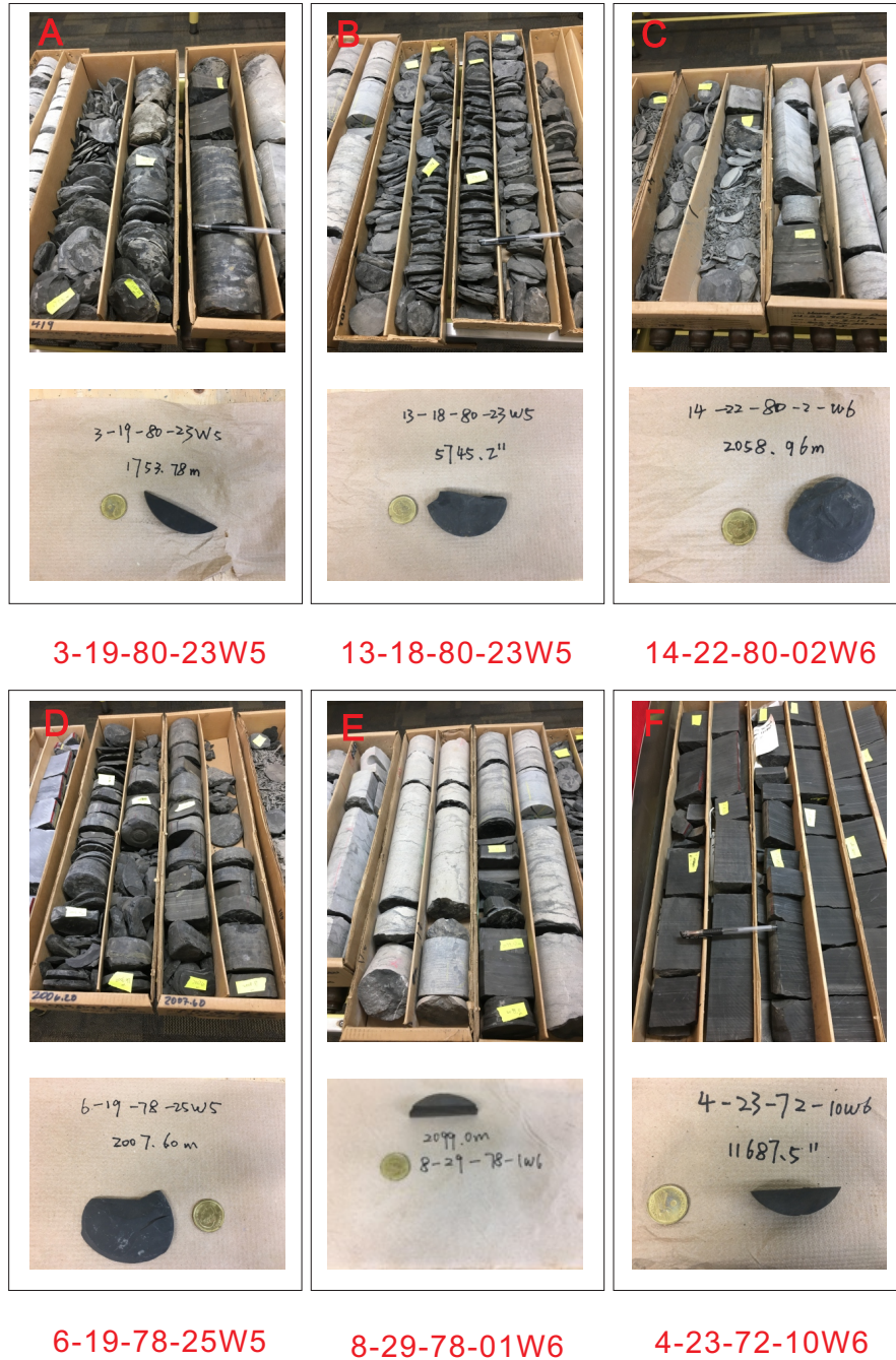
Fig. 6. Drill cores for the Exshaw Formation and representative black shale samples for each core. Drill cores 3-19-80-23W5 (A) and 13-18-80-23W5 (B) are in the immature zone. Drill cores 14-22-80-02W6 (C), 6-19-78-25W5 (D), and 8-29-78-01W6 (E) are in the mature zone. Drill core 4-23-72-10W6 (F) is in the overmature zone.
