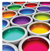
Figure 02.35 • Acrylic Comes in many forms ranging from sheet goods to liquid applied paints. Can be clear to opaque, and can be quite strong in its rigid form.
