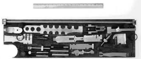
Figure 03.7 • Ordnance Department Inspection Gauge Inspection gauge for the Mississippi Rifle model 1941, by Eli Whitney Jr.
