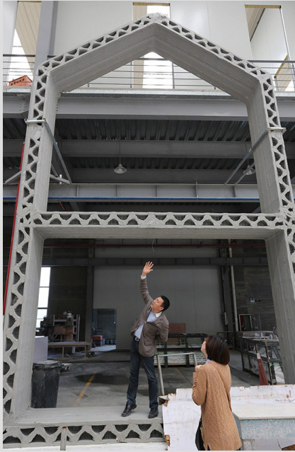
Figure 01.40 • Prototype with two storey frame
