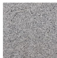
Figure 02.25 • Granites An igneous rock, formed by solidification of the earth's magma. Hard and dense, thus durable, water impenetrable, impact resistant, and stable in tough environments. It comes in many finishes such as polished, flamed, honed.
