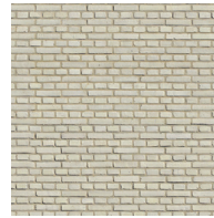
Figure 02.20 • Clay Brick Durable and Strong - load bearing walls, screens, structure, finishing int./ext., floors, roadways, modular, comes in many shapes/sizes/textures/colours.
