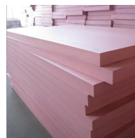
Figure 02.32 • Expanded Polystyrene In its expanded form polystyrene is rigid and does a good job of preventing thermal transmittance.
