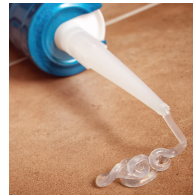
Figure 02.30 • Silicone Sealant - Creates a thermal, water, air, and vapour barrier. Structural - used for its high setting strength which allows it to hold objects in place securely such as glazing in curtain walls.
