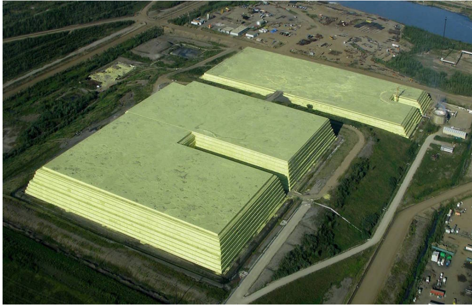
Figure 1.1: Sulphur removed from crude at Suncor operation, Fort McMurray. Alberta alone produced 3.9 million tons of sulphur in 2017 [2, 3].
