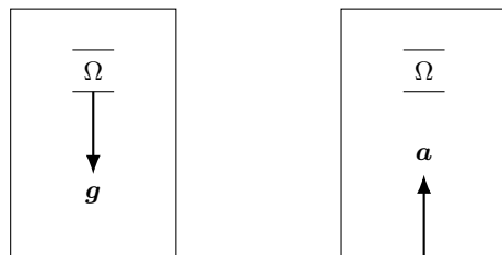
Figure 3.2: Quantum WEP setup: a two-level atomic ‘detector’ with gap \Omega (with respect to its proper frame) in a cavity. The cavity contains a quantum field whose modes may lead to atomic excitations (even in the vacuum state), and hence detector responses. The atom serves as a detector in the sense that a particle is detected when the atom is excited and then emit radiation [3].
