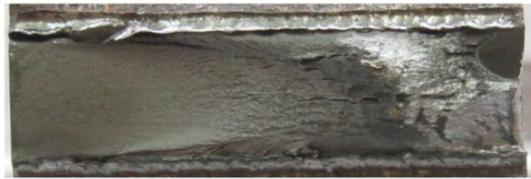
Figure 4.34: Fracture surfaces for HFMI treated 350W steel specimens under CA loading
