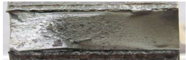
Figure 4.34: Fracture surfaces for HFMI treated 350W steel specimens under CA loading
