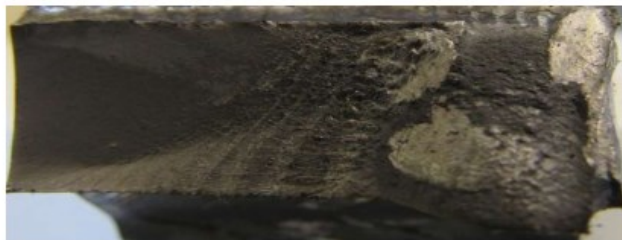
Figure 4.58: Fracture surfaces for HFMI treated A514 steel specimens under CA-UL loading
