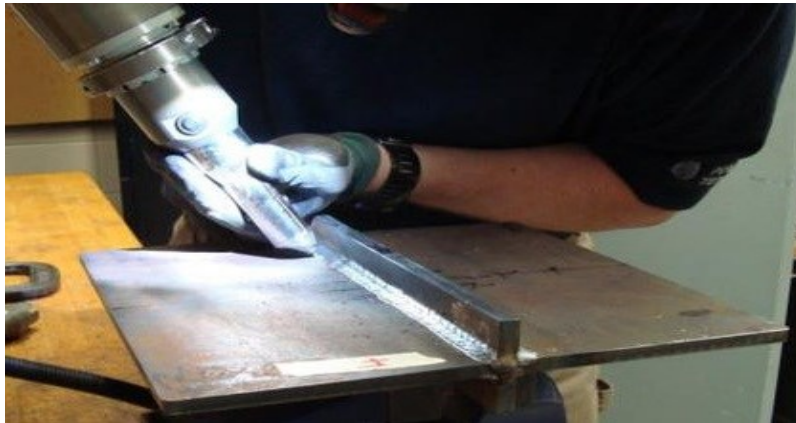
Figure 4.1: HFMI treatment of 12" long high strength steel weld
