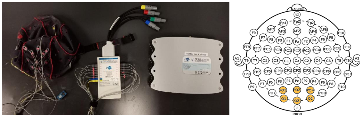
Figure 2.3. Data Acquisition hardware illustrating the EEG cap with the g.Scarabeo electrodes, the g.GammaBox driver and g.USBamp Amplifier. 10-20 system based electrode montage depicting O1, O2, Oz, PO3, POz, PO4.
