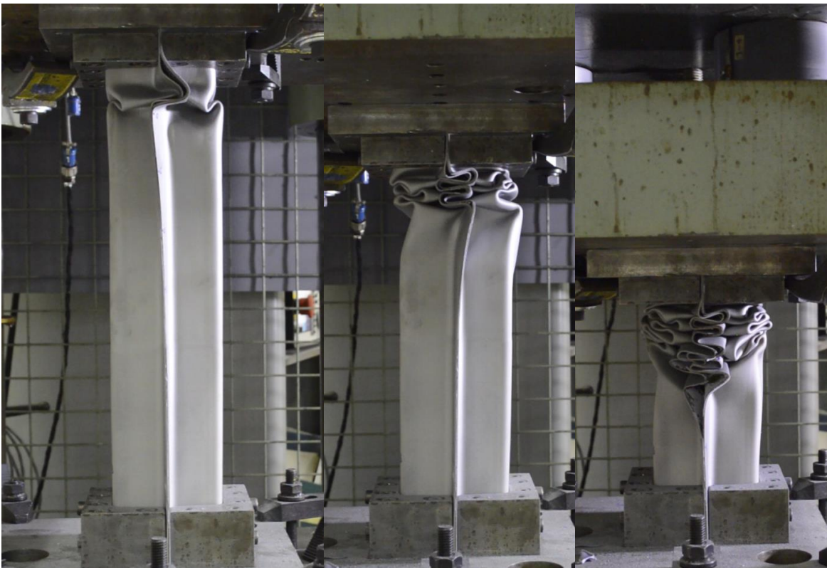
Figure 5.19: QS-AX-3Z-GB specimens demonstrating folding deformation during quasi-static axial crush experiment, with very minimal flange separation
