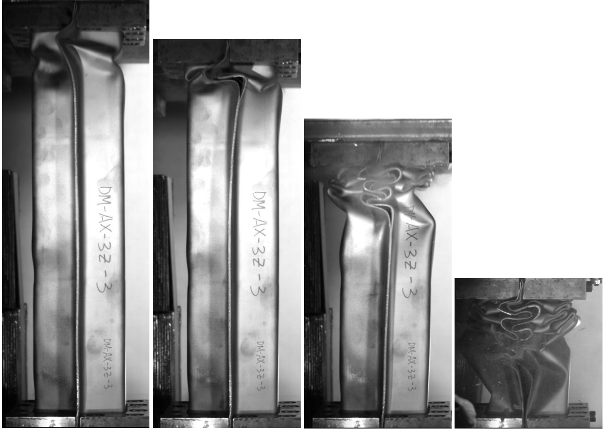
Figure 6.20: DM-AX-3Z-GB model Deformation mode with Omer’s (2014) predicted hardness (top row) and that of manually assigned hardness mapping corresponding to the measured values in the current work (middle row), showing a deformation pattern that correlates much better with the experiment (bottom row)
