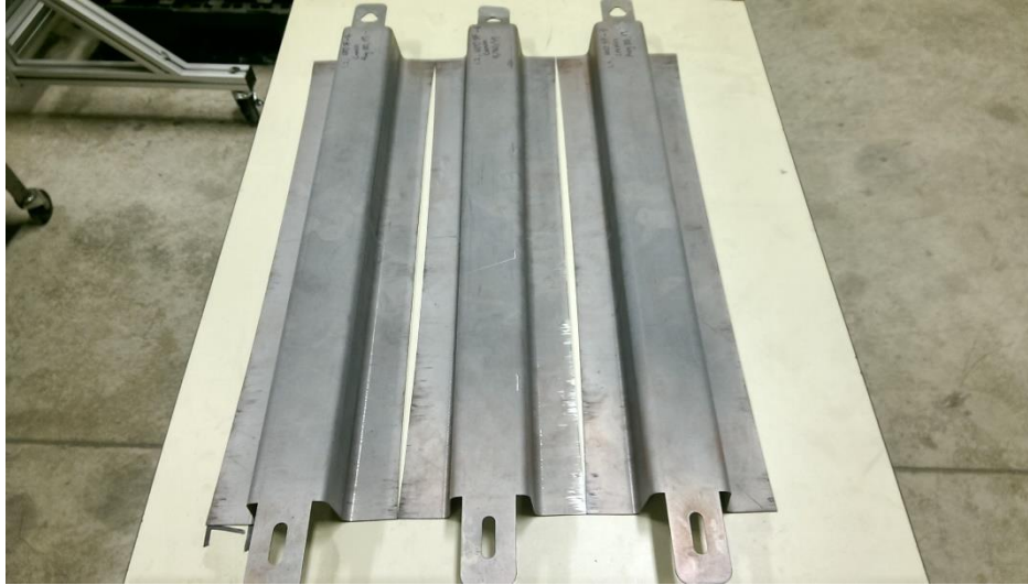
Figure 3.18: Gap between flanges of soft flange samples when placed side by side
