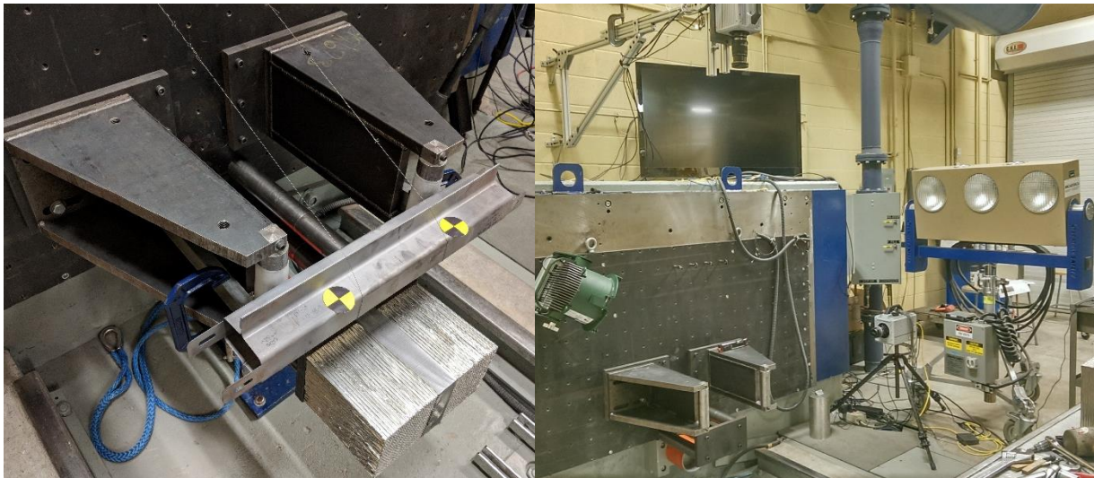
Figure 3.29: Dynamic three-point bend experimental setup, showing the mounted specimen, honeycomb packs, and cameras
