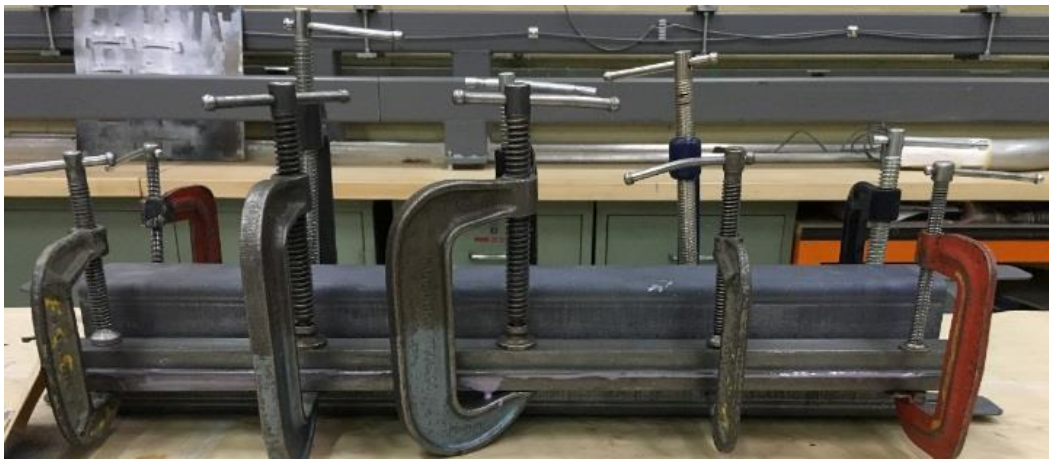
Figure 3.16: C-clamps used to secure the flange prior to curing the assembly in the oven
