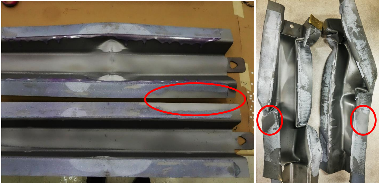
Figure 3.19: Failure surface of early quasi-static fully martensitic three-point bend (left) and axial crush (right), showing inconsistent adhesive coverage
