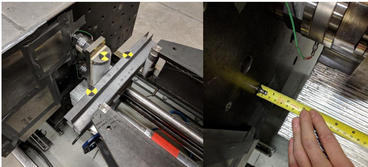
Figure 3.30: Sled and impactor brought in contact with the specimen to demonstrate distance of free crush zone
