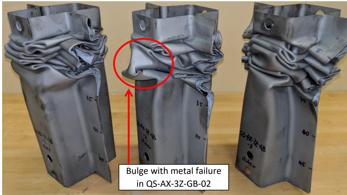
Figure 5.20: Final deformed state of QS-AX-3Z-GB specimens, note that the bulge with metal failure in QS-AX-3Z-GB-02 was caused by fixture slippage
