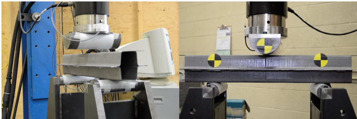
Figure 3.22: Quasi-static three point bend experimental setup
