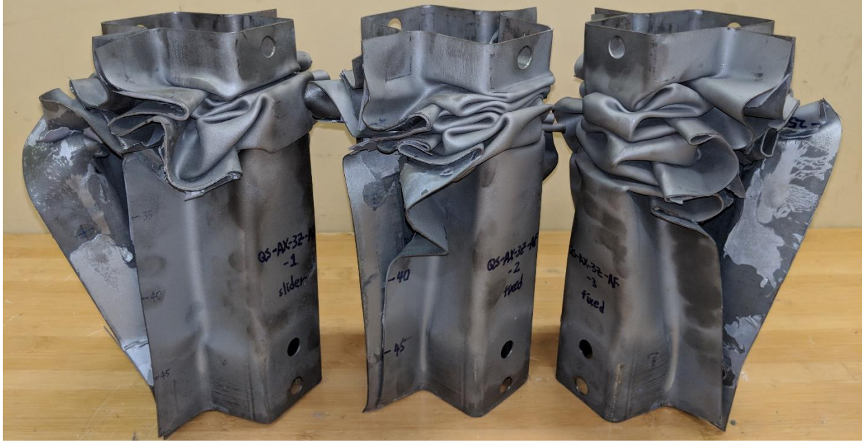
Figure 5.23: Final deformed state of QS-AX-3Z-AF specimens, showing extensive flange separation and interfacial adhesive failure
