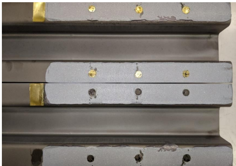
Figure 5.36: Failure surface of fully martensitic Caiman samples, showing consistent and uniform adhesive coverage
