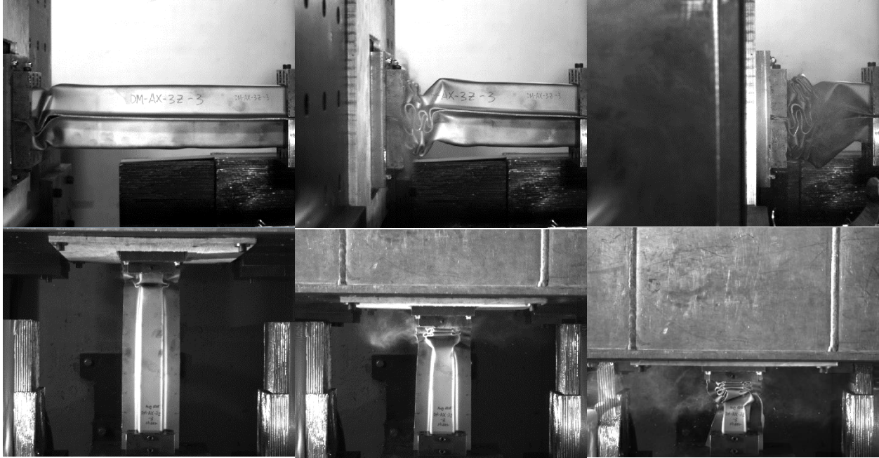
Figure 5.30: Stable and controlled collapse in DM-AX-3Z-GB-03, showing fold initiation at the indent (left), and extensive fold development (center and right)
