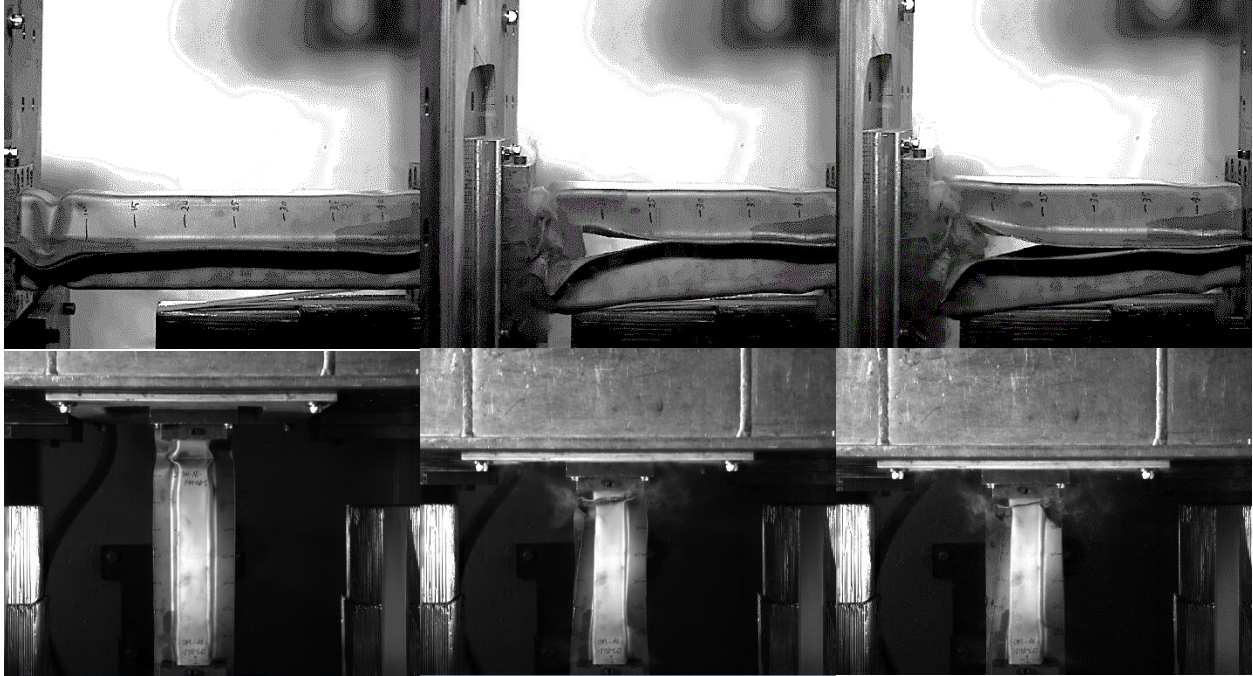
Figure 5.26: Global buckling deformation mode in DM-AX-FM-GB-01, showing fold initiation (left), and rapid crack propagation (center and right)
