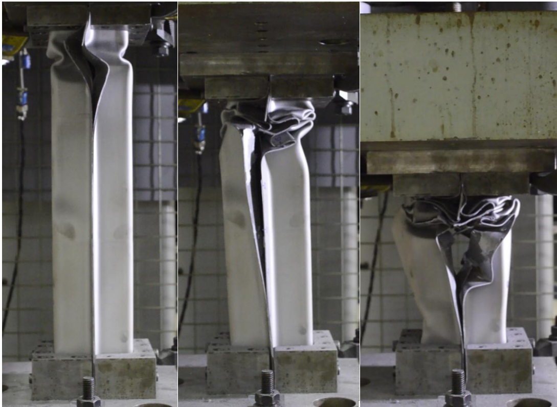
Figure 5.22: Deformation mode of QS-Ax-3Z-AF specimens, initiating with folding then transitioning to global buckling due to extensive flange separation
