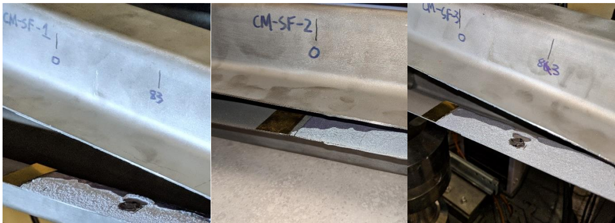
Figure 5.35: Areas of unbonded adhesive due to the curvature of soft flange hat sections, making it difficult to fully clamp down the center along the length of the tube
