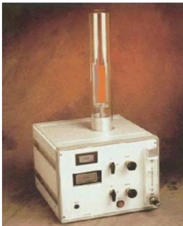
Figure 2.12: General view of the limiting oxygen index apparatus
