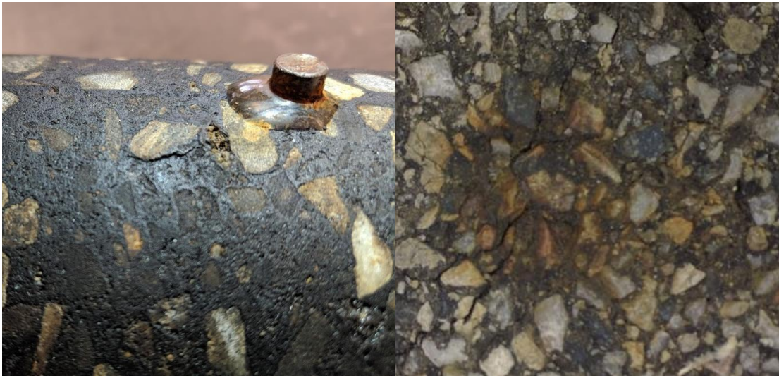
Figure 8-1 The Initiation of Cracks Around the Activated Iron Sulphide Containing Aggregates in (a) Laboratory Conditioned Sample (b) on The Surface of Pavement
