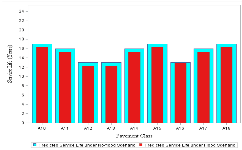
Figure 4-16 Estimated Service Life of Pavement Classes (A10-A18) under High Traffic Conditions
