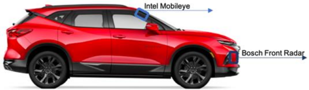
Figure 38: Side view of front sensor placement on Chevrolet Blazer
