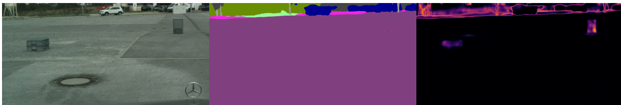
Figure 1.1: Image from the LostAndFound dataset [38], where two unlikely objects (storage crates) are almost entirely incorrectly predicted to be road. The Max Softmax method – described in detail later – clearly highlights these crates as OOD. (best viewed in colour)
