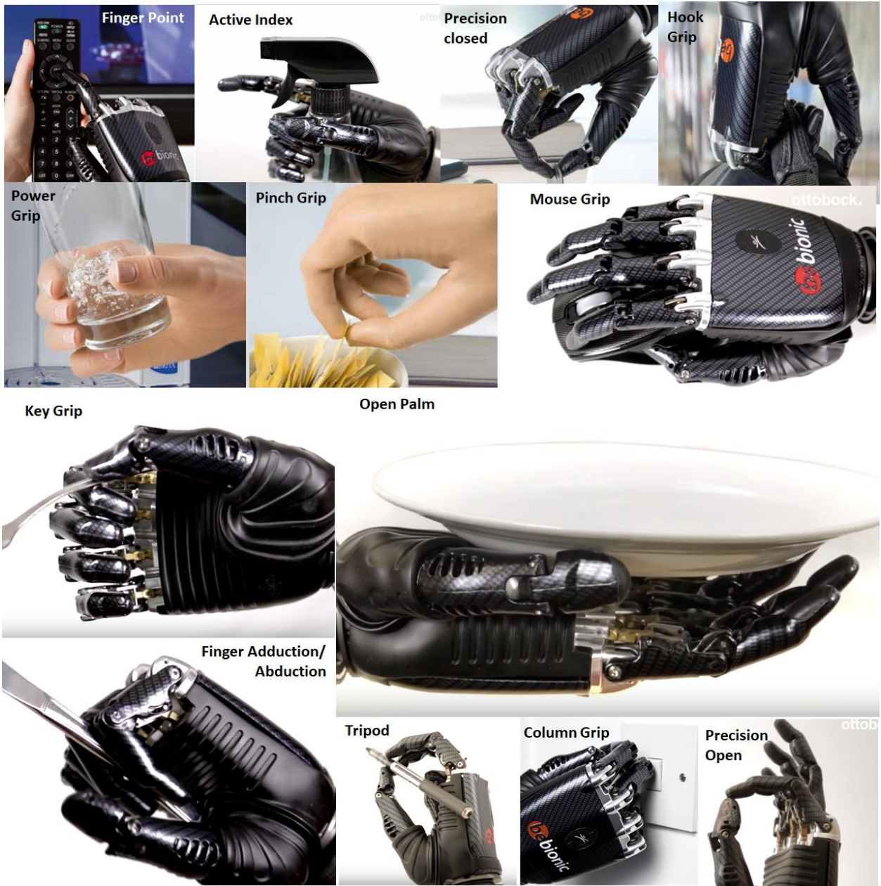
Figure 8.1, this figure depicts the 13 gestures available for use with the Bebionic V3 hand prosthesis developed by Ottobock. The “rest” gesture was omitted as it is not actively used for grasping or manipulation tasks
