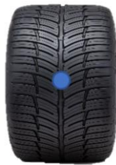
Figure 2 - Point mass representation; a single lumped mass with a tire acting as the limiting factor in providing grip.
