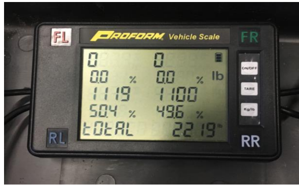
Figure 26 - Measurement of the weight seen at the un-lifted wheels during testing
