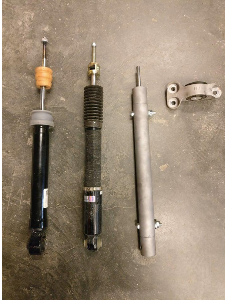
Figure 23 - Side by side comparison of the stock rear damper, aftermarket rear damper, and solid damper used for testing
