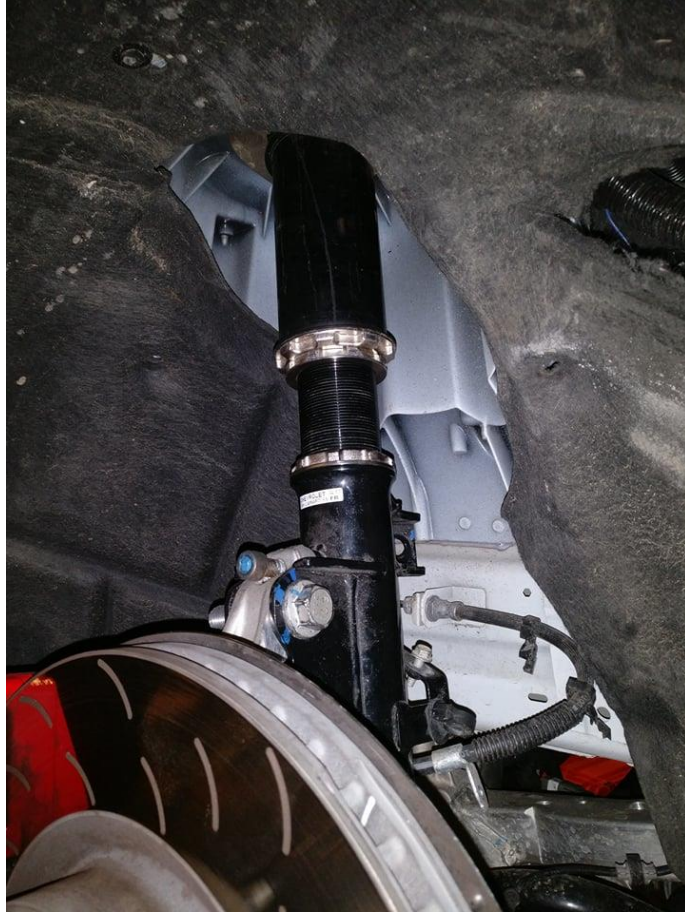
Figure 21 - Front suspension with "solid" spring to prevent suspension articulation during testing process
