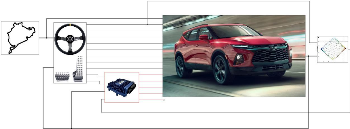
Figure 33 - Top level overview of Simulink model. From left to right: road profile, driver block, vehicle dynamics controller, vehicle model, visualization block. Blazer image [23]
