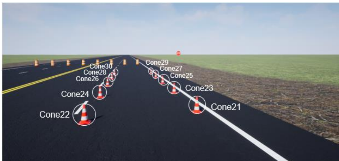
Figure 47 - Cones defined in the Unreal Engine virtual environment for a double lane change test case [36]
