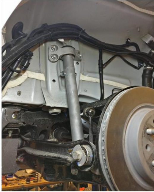
Figure 22 - Rear suspension fixture for preventing suspension travel during CGH testing
