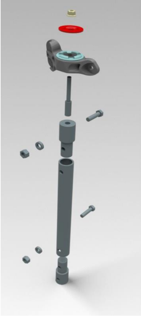
Figure 22 - Rear suspension fixture for preventing suspension travel during CGH testing
