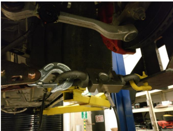
Figure 30 - Suspension compliance testing device being used on the front suspension
