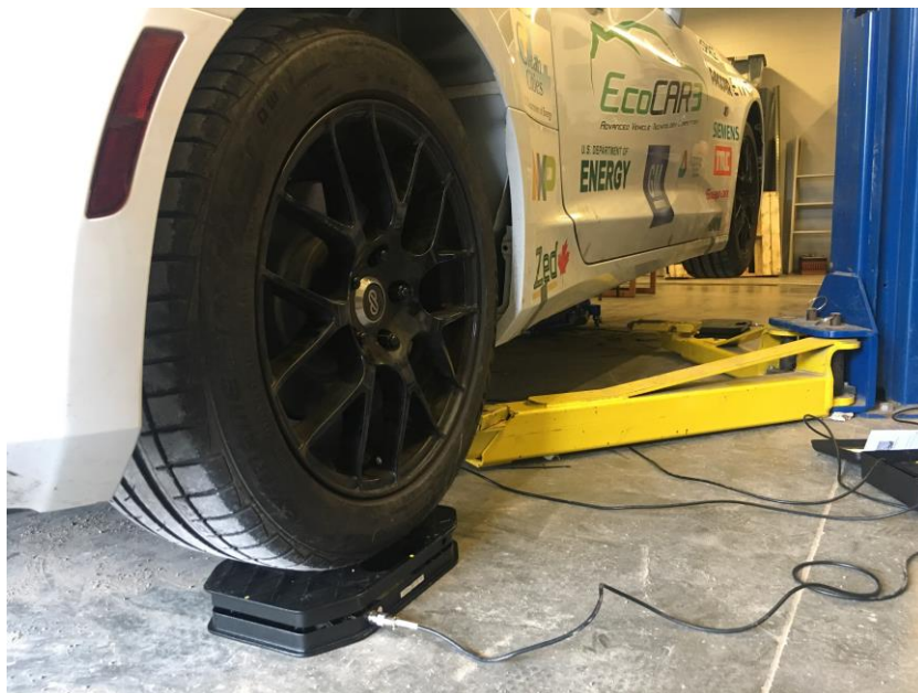
Figure 25 - Lifting the vehicle to measure the weight transfer to the un-lifted wheels to measure CGH
