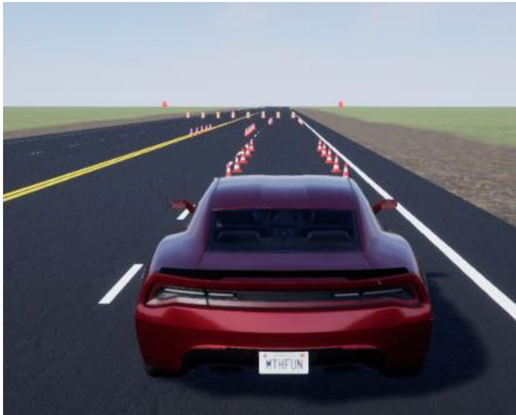
Figure 46 - Double Lane change test case, visualized using the Unreal Engine [36]
