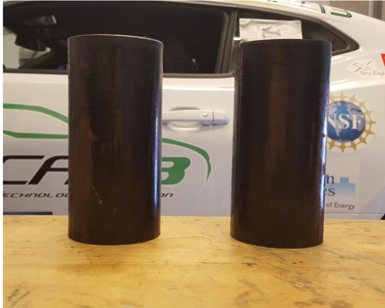
Figure 20 - Custom spring replacements for the front suspension were fabricated and used to prevent suspension travel during CGH testing
